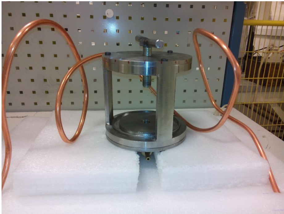
Fig. 17 O-rings compressor surrounded by copper wire.
