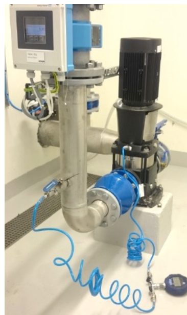
Figure 3.2.4: Pressure reading arrangement for check valve
