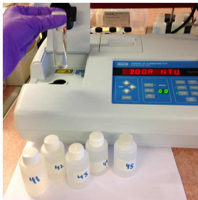
Figure 5-12: Turbidity measured with a turbidimeter
