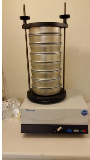
Figure 72 The machine and sieves used for the analysis. (Photo: Jens H. Trandem)
