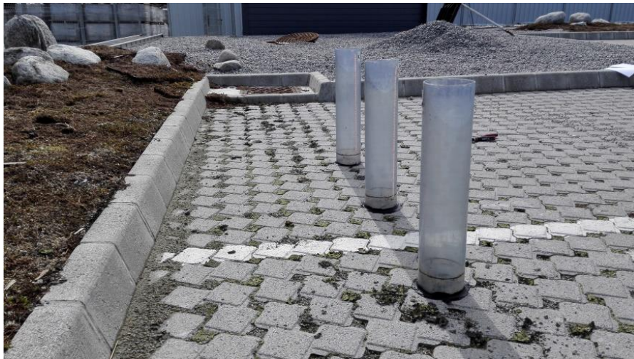
Figure 63 Test 1 at the lower part of the pavement. (Photo: Jens H. Trandem)
