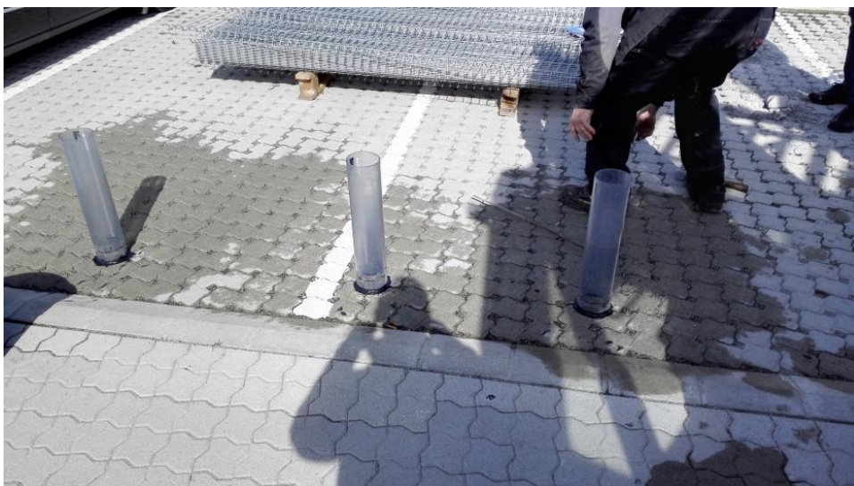
Figure 65 Test 3 from the upper part of the permeable pavement in test area 3. (Photo: Jens H. Trandem)
