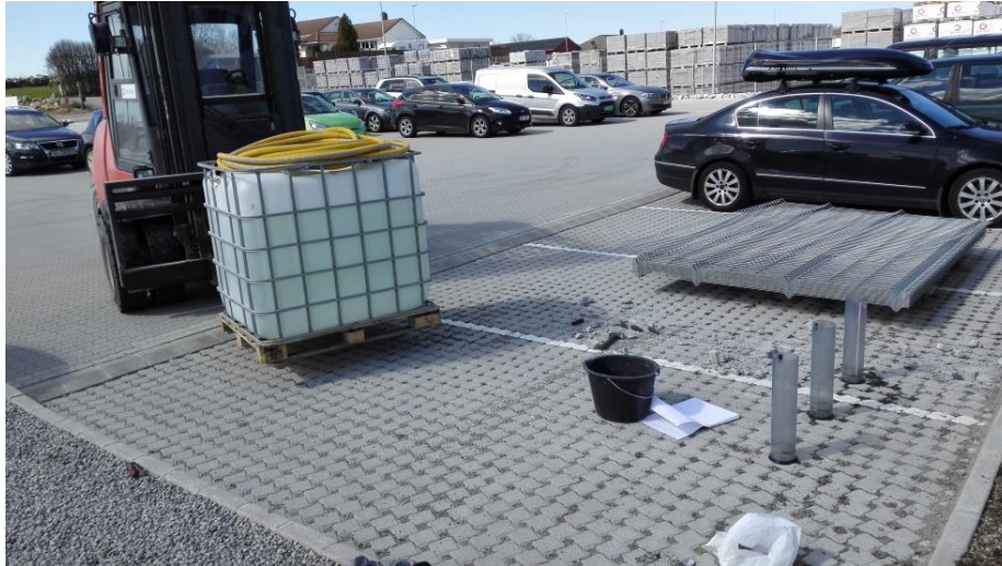
Figure 67 Overview of the area and infiltration tests (Photo: Jens H. Trandem)
