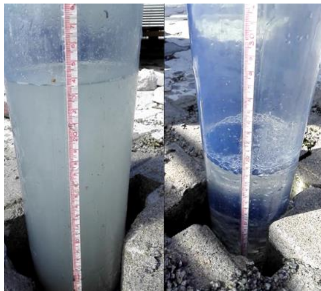
Figure 70 Left: Test 2 MPD 2 Trial 1. Right: Another test done for the bedding layer. The difference in water quality with regards to fine particles and dust is significant. (Photo: Jens H. Trandem)
