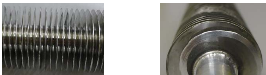
Figure 3-10: Pictures of the aluminium finned tubes–Geometry 8. Left: view from the side; right: view of the fins
