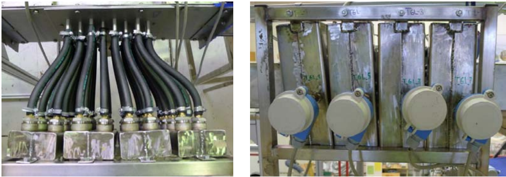
Figure 3-6: Turning chambers mounted in a frame. Left: connection between the finned tubes and the turning chambers with hoses; right: turning chambers and temperature sensors
