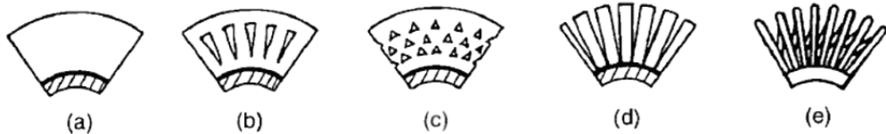
Figure 2-1 Enhanced circular fin geometries. (a) plain circular fin, (b) slotted fin, (c) punches and bent triangular projections, (d) serrated fin and (e) wire loop extended surface [Webb and Kim (2005)]
