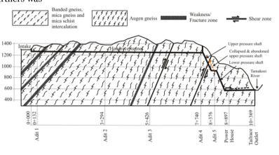
Figure 4: Geology along the waterway system of Khimti I Hydropower Project
