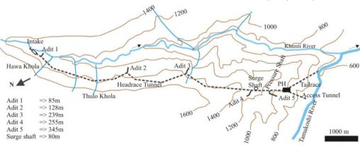
Figure 2: The layout arrangement of Khimti I Hydropower Project
