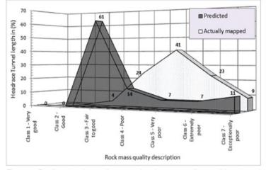
Figure 5: Predicted and actually mapped rock mass quality condition along the Since only 18 m shaft excavation was remaining, headrace tunnel.
