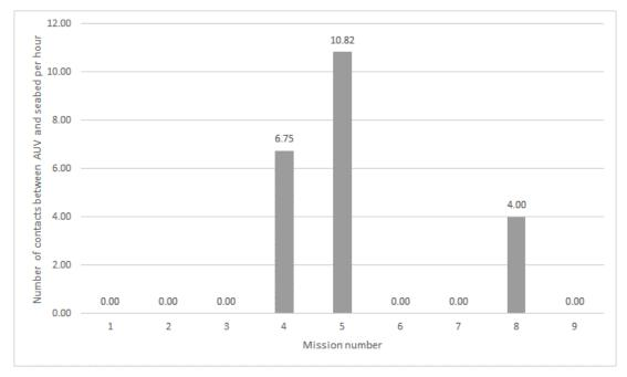
Figure 5 Number of contacts between AUV and seabed per hour of operation, recorded during nine missions of the REMUS 100 of the NTNU AUR Lab between 06. August 2015 and 19. November 2015.
