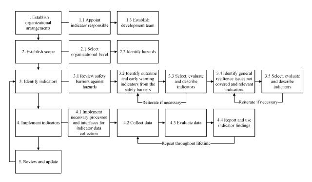
Figure 1 Steps in the synthesized process for developing safety indicators for AMS, based on [20, 66]
