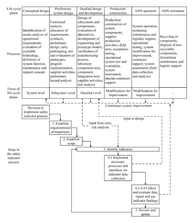
Figure 2 The process for developing safety indicators in relation to the system life cycle of an AMS (system lifecycle adapted from Blanchard [4], figure 1.12). Solid lines represent the sequential order of steps. Dashed lines represent feedback and feedforward of information and initiation of reiterations.
