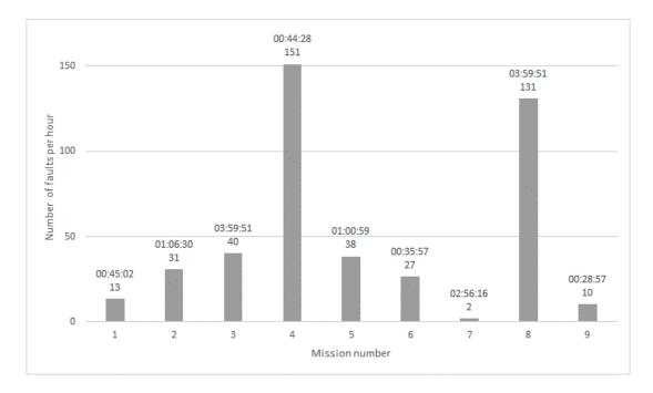
Figure 4 Number of faults per hour of operation recorded during nine missions of the REMUS 100 of the NTNU AUR Lab between 06. August 2015 and 19. November 2015. Total mission time is displayed above the number of faults.
