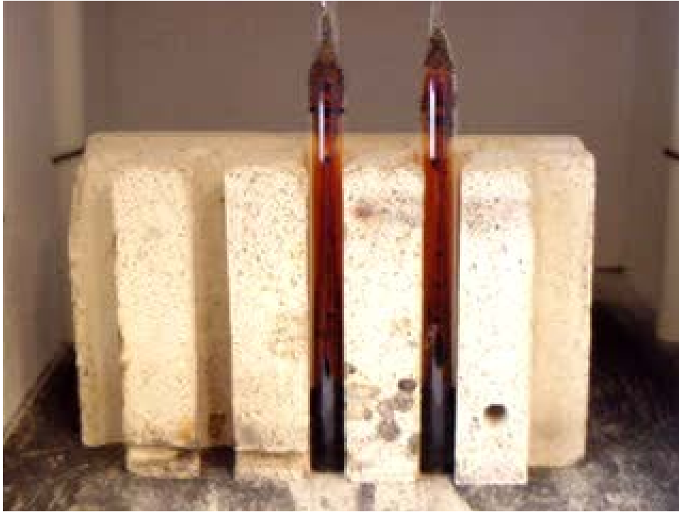
Figure B-2 The sealed ampoules in the lab oven at 550°C
