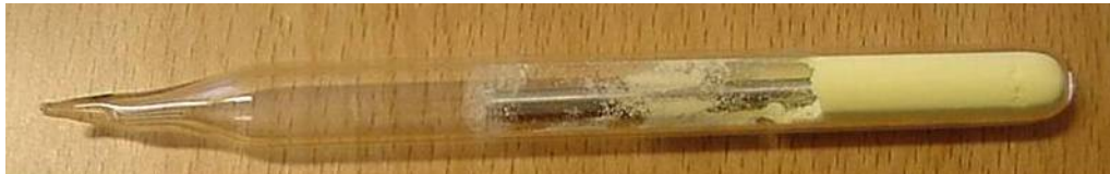
Figure B-1 Sealed silica glass ampoule containing sulfur and metal rod
