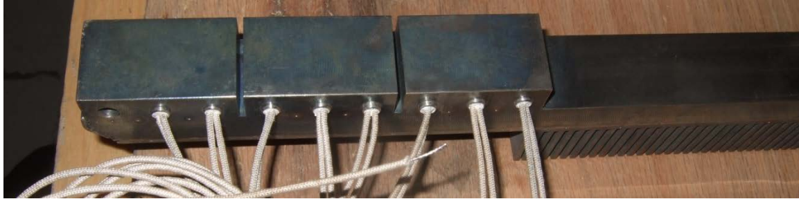
Figure 3-19 The hybrid heat pipe with the heater cartridges
