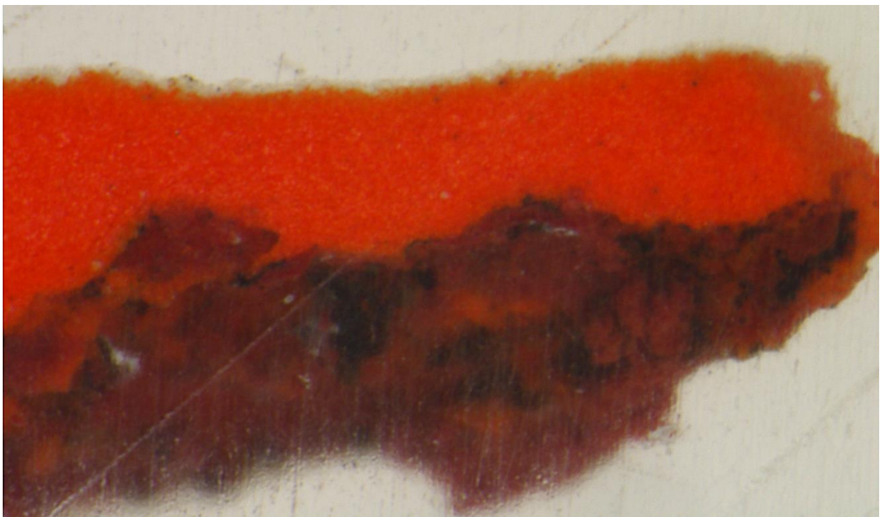
Figure 32. Red paint sample from Bardal rock art site displaying multiple paint applications (11X magnification)
