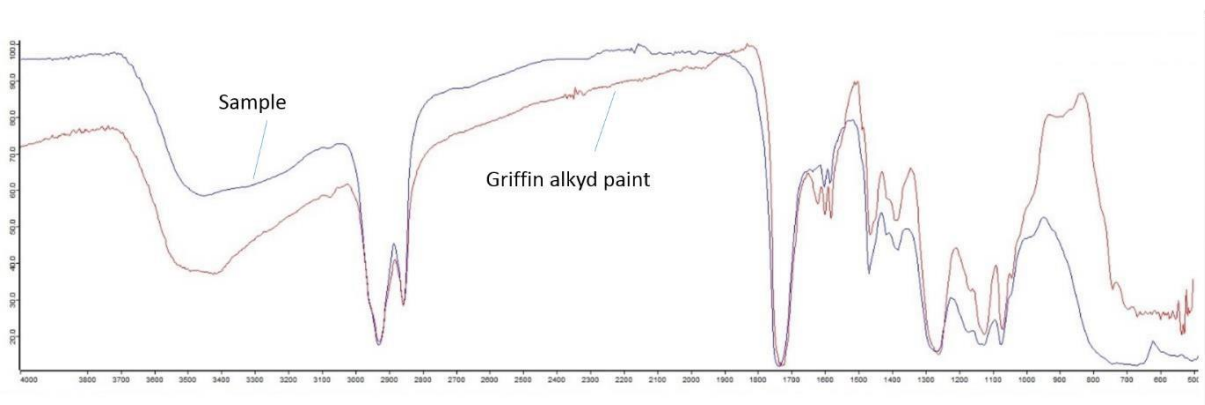
Figure 59. IR spectrum of a sample of yellow paint between yellow and red paints from Hell rock art site and that of a Griffin alkyd paint
