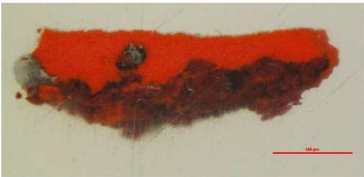
Figure 9. Red paint sample from Bardal rock art site displaying multiple paint applications (5x magnification)
