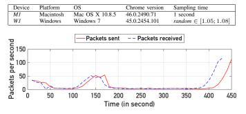
Figure 2: Packet transfer rate (sender *M1* to receiver *W1*)
