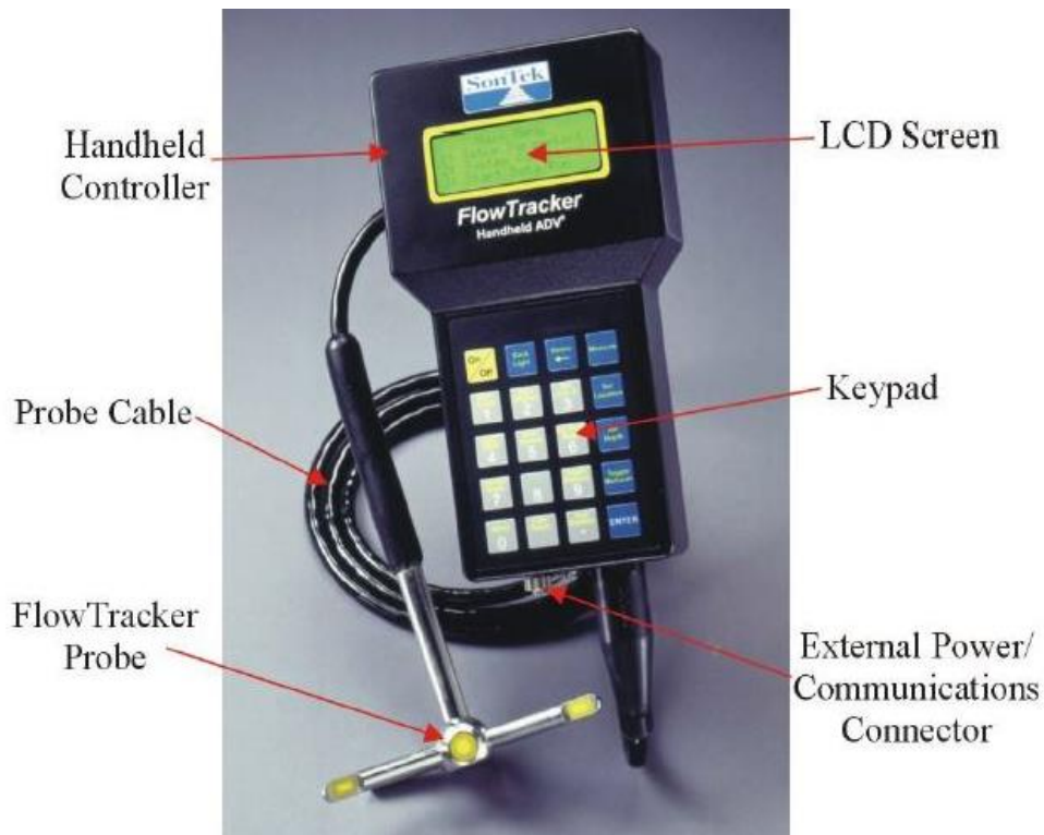
Figure 3-2. Major components of Flow Tracker. ( www.sontek.com , 2007)
