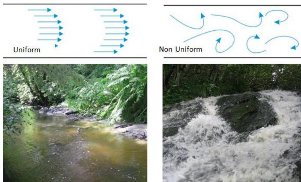
Figure 3-6. Description of proper place for Logger installation from the flow regime point.
