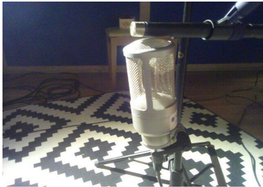
Picture 2.2.1 – The positioning of the Ehrlund EHR-M and the DPA4090 together about 45 cm from the cello. The carpet is there to prevent additional floor reflections.
