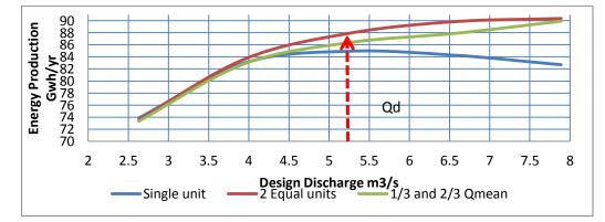
Figure 25 Turbine Optimization Result for Single unit, 2unit of Equal capacity and 1/3&2/3 Q <sub>mean</sub>
