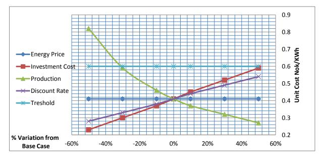
Figure 37 Sensitivity Analysis: Unit Cost against Variation
