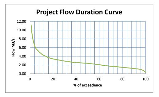
Figure 14 Flow duration curve project catchment FDC
