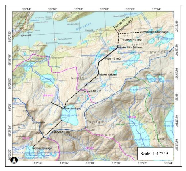
Figure 9 Project Layout plan Source: Gislink.no
