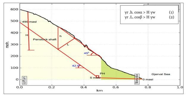
Figure 23 Limit Equilibrium method: Design for Minimum Rock Cover
