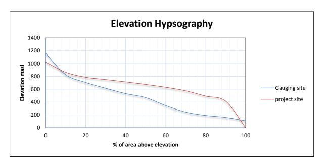
Figure 10 Hypsographic curve of Vassvatnet and Project site
