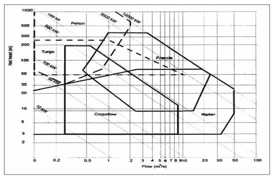
Figure 4 Guide Curve for Turbine Type Selection
