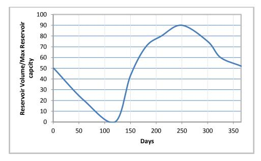
Figure 27 Reservoir Rule Curve: Source (Killingtivet, 2000)
