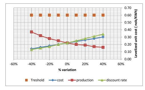
Figure 6 sensitivity of unit cost against variation Scheme 10
