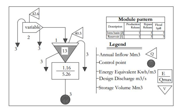
Figure 28 Layout of nMag2004 setup for the power plant system
