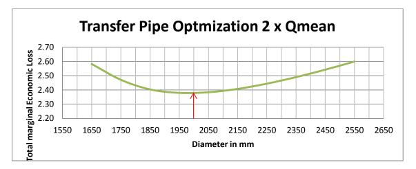
Figure 22 Pipe Optimization 2x Q mean
