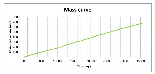
Figure 11 Mass curve for gauging station at Vassvatnet
