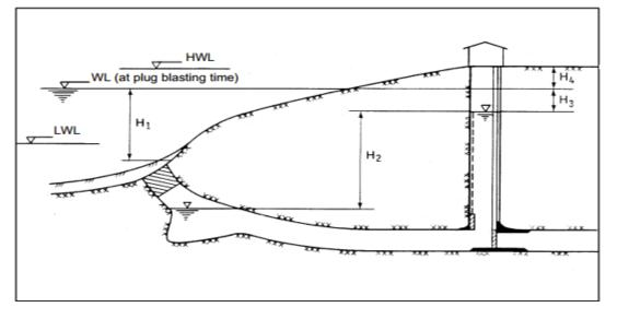
Figure 20 Open System Piercing, Geometric layout of intake Source: (Bruland, 2000)
