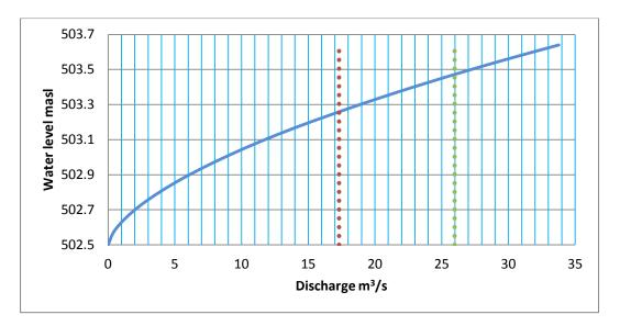
Figure 19 Rating Curve over the Spillway
