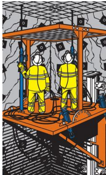
Figure 40 Alimak working platform (Hardrockminerclothing, 2014)
