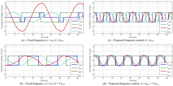
Fig. 10. Comparison between IPT voltages and currents at rated power and different coupling for two different design and control methods
