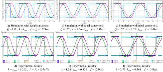
Fig. 13 Comparison between simulations and experiments in different coupling conditions; IPT system operated at rated I/O voltage and variable frequency, to achieve rated output power. The curves show: Blue (solid): *V<sub>send</sub>* (25 V/div), Cyan (dashed): *V<sub>pick</sub>* (25 V/div), Green (solid): *I<sub>send</sub>* (5 A/div), Purple (dashed): *I<sub>pick</sub>* (5 A/div)
