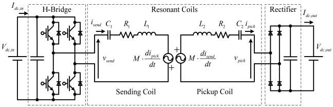
Fig. 1. Selected topology for IPT system with dc-source and CVL
