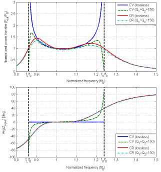
Fig. 5. Comparison between characteristics of SS- IPT system with optimally matched CR load at resonant frequency according to (19) and with CV load corresponding to  $x_u = 1$ , at k = 0.35
