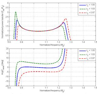
Fig. 7. Effect of capacitance detuning on IPT characteristics; Coils with k = 0.35,  $Q_1 = Q_2 = 150$  and unbalanced with  $x_u = 0.95$
