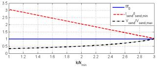
Fig. 3. Variation of sending voltage and current as function of coupling, assuming rated power flow and operation in resonance
