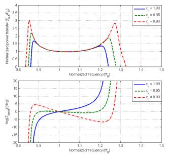
Fig. 6. Effect of design unbalance on IPT characteristics; Coils with k = 0.35,  $Q_1 = Q_2 = 150$ .
