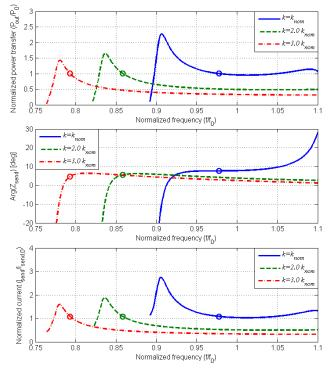
Fig. 8. IPT characteristics and operating points (marked with circles) at rated power, constant *I/O* voltage, variable coupling; Coils with  $k_{nom} = 0.2$ ,  $Q_1 = Q_2 = 150$ ;
