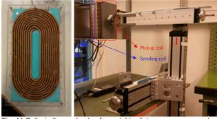
Fig. 11 Coil winding and setup for variable-distance measurements.
