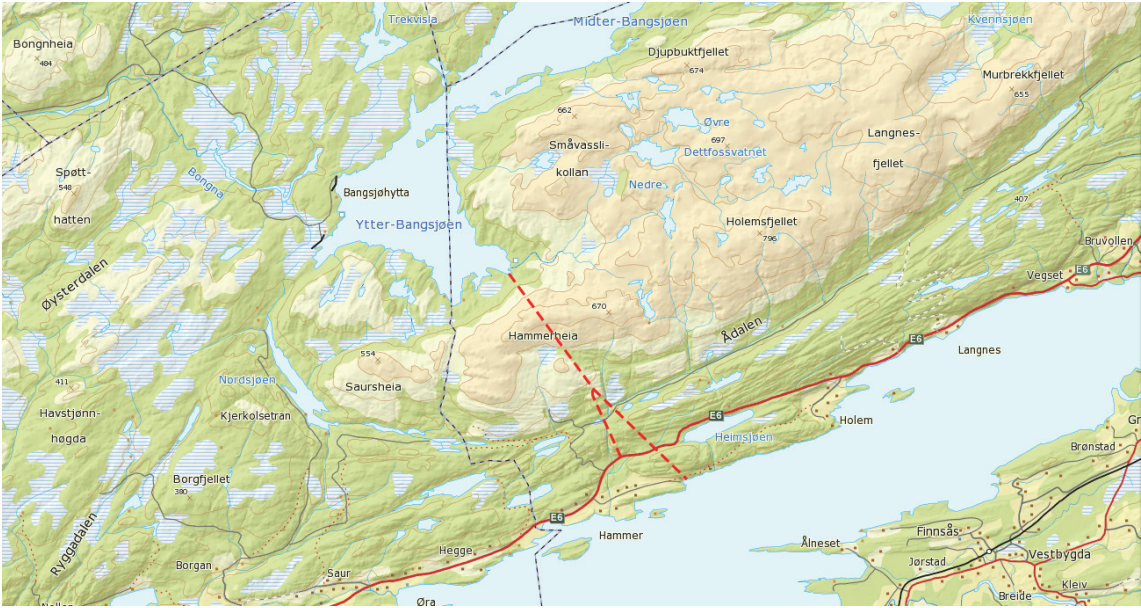
Figure 4.2 Topographic map with tunnel alignment
