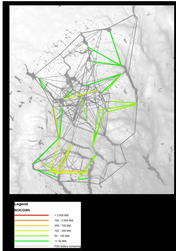
Figure 15: Figure 14: PSH connections suggested by the tool for P-14 classified by the NOK/GWh
