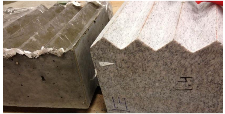
Figure 75. Plastic adhesive to avoid bonding (ii).
