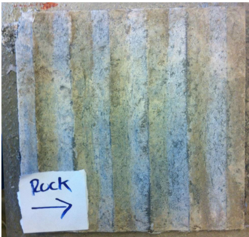
Figure 142. Test 3.2 Rock interface after the test is finished.
