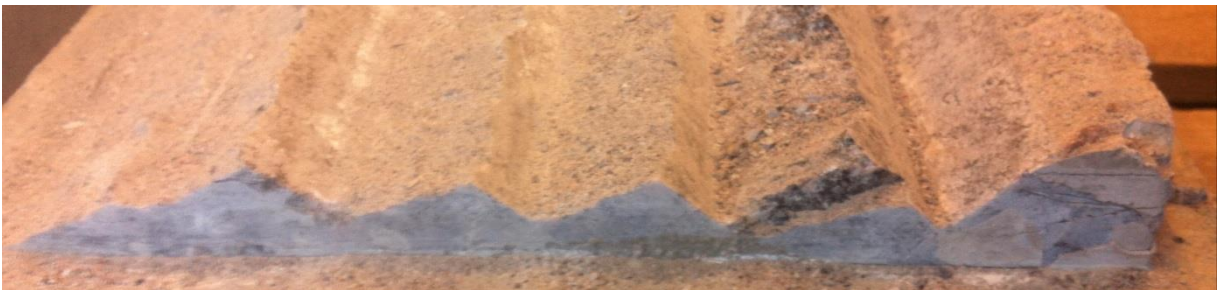
Figure 106. Test 1.1 Rock asperities profile after the test.
