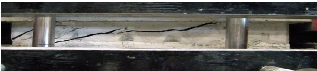
Figure 49. Failure for the specimens tested with bonding for i=40^\circ and \sigma_n = 1.2 \text{ MPa} .
