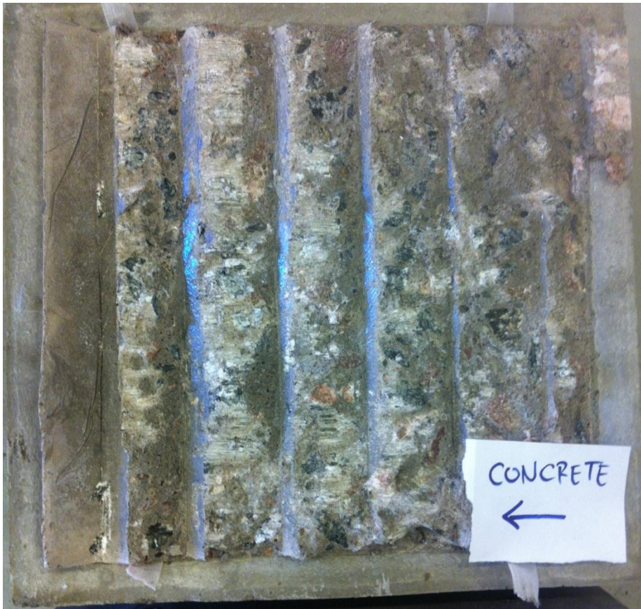
Figure 113. Test 1.3 Concrete interface after the test.
