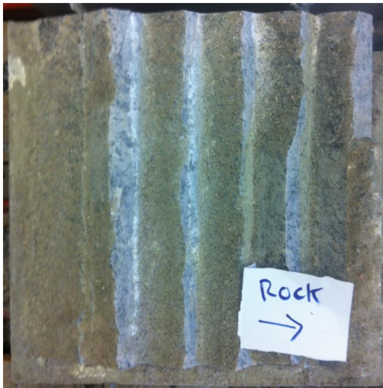
Figure 102. Test 1.1 Rock interface after the test.
