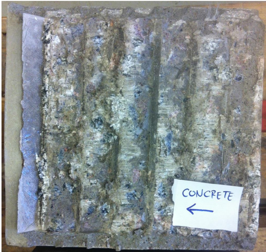
Figure 120. Test 1.4 Concrete interface after the test.
