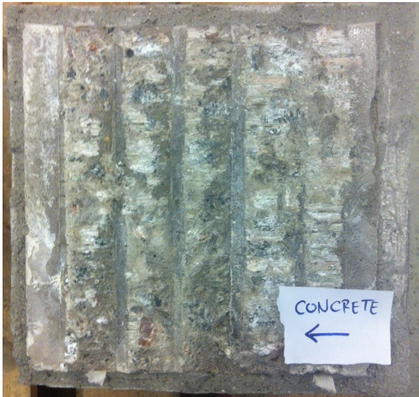
Figure 134. Test 2.3 Concrete interface after the test.
