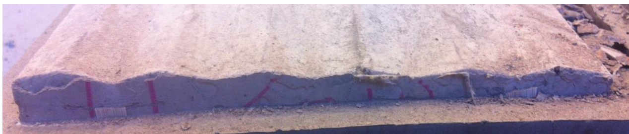
Figure 146. Test 3.2 Rock asperities after the test.
