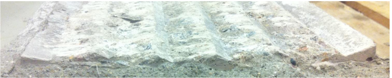
Figure 136. Test 2.3 Concrete asperities profile after the test.
