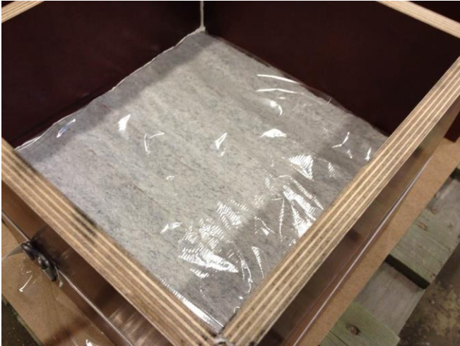
Figure 76. Plastic adhesive to avoid bonding (i).
