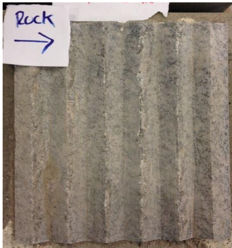
Figure 126. Test 2.1 Rock interface after the test.
