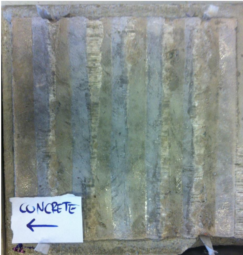
Figure 149. Test 3.3 Concrete interface after the test.
