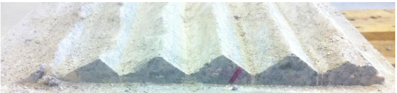
Figure 121. Test 1.4 Rock asperities after the test.
