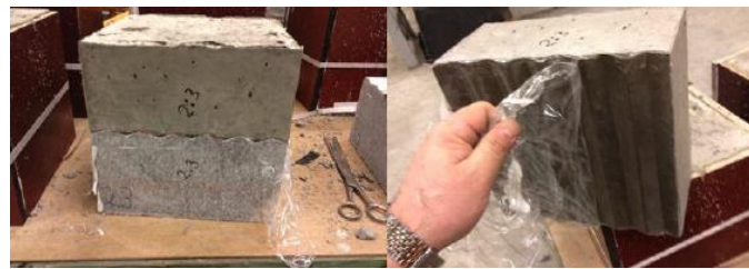
Figure 35. Formwork removed from rock sample and plastic wrap being removed (taken from (Liahagen, 2012))
