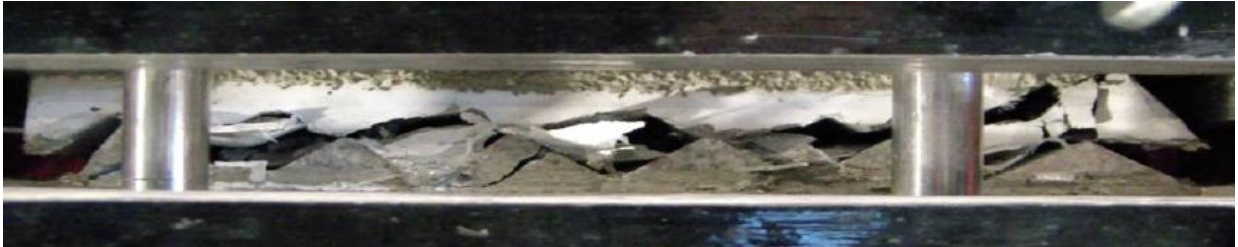
Figure 53. Test 1.1 Concrete-to-rock interface after the test is finished (taken from (Liahagen, 2012)).
