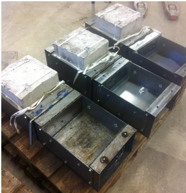
Figure 77. Casting on the steel molds (i).
