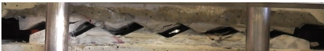
Figure 83. Test 2.3 asperities failing.
