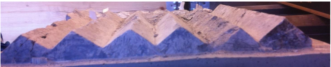
Figure 115. Test 1.3 Rock asperities profile after the test.
