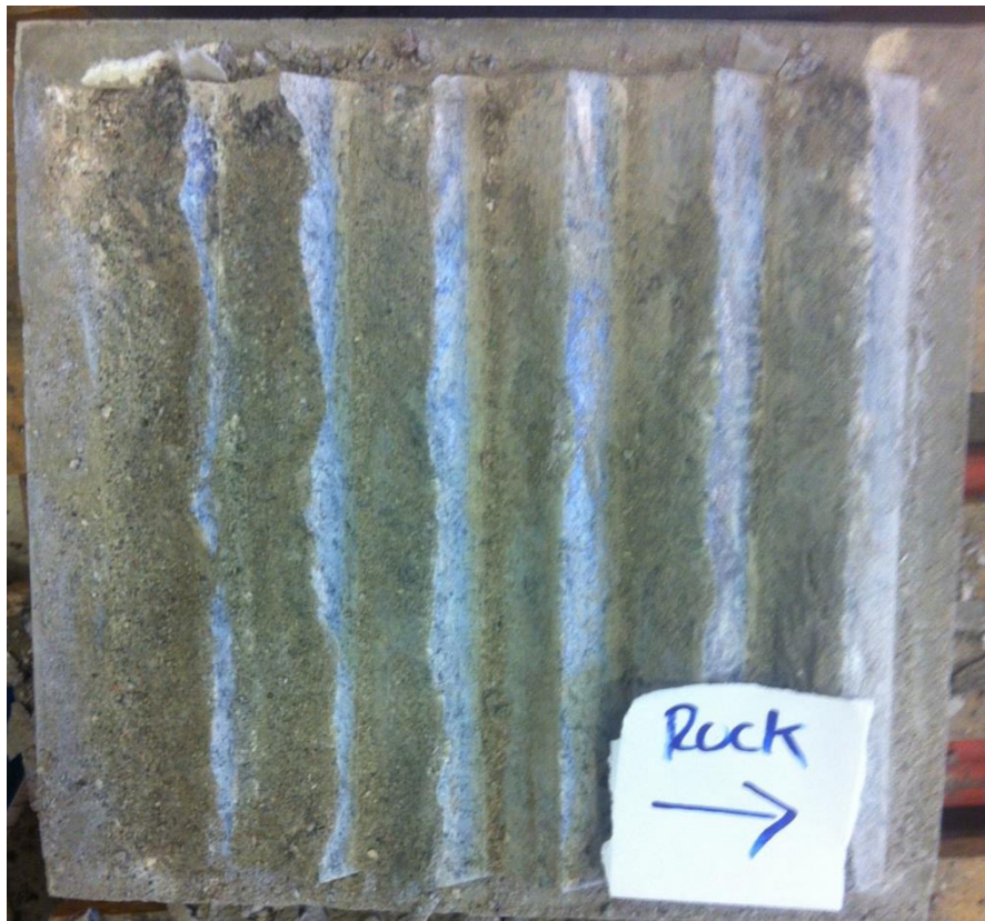
Figure 119. Test 1.4 Rock interface after the test.
