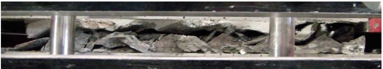
Figure 54. Test 1.2 Concrete-to-rock interface when peak shear stress is reached (taken from (Liahagen, 2012)).
