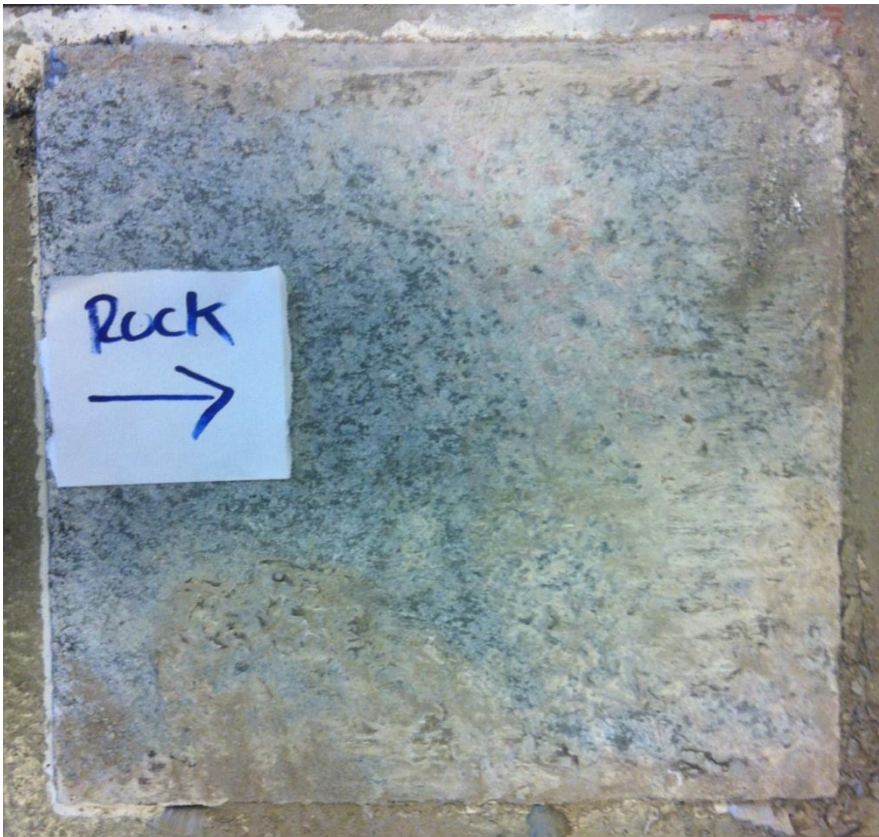
Figure 159. Test 4.2 Rock interface after the test.
