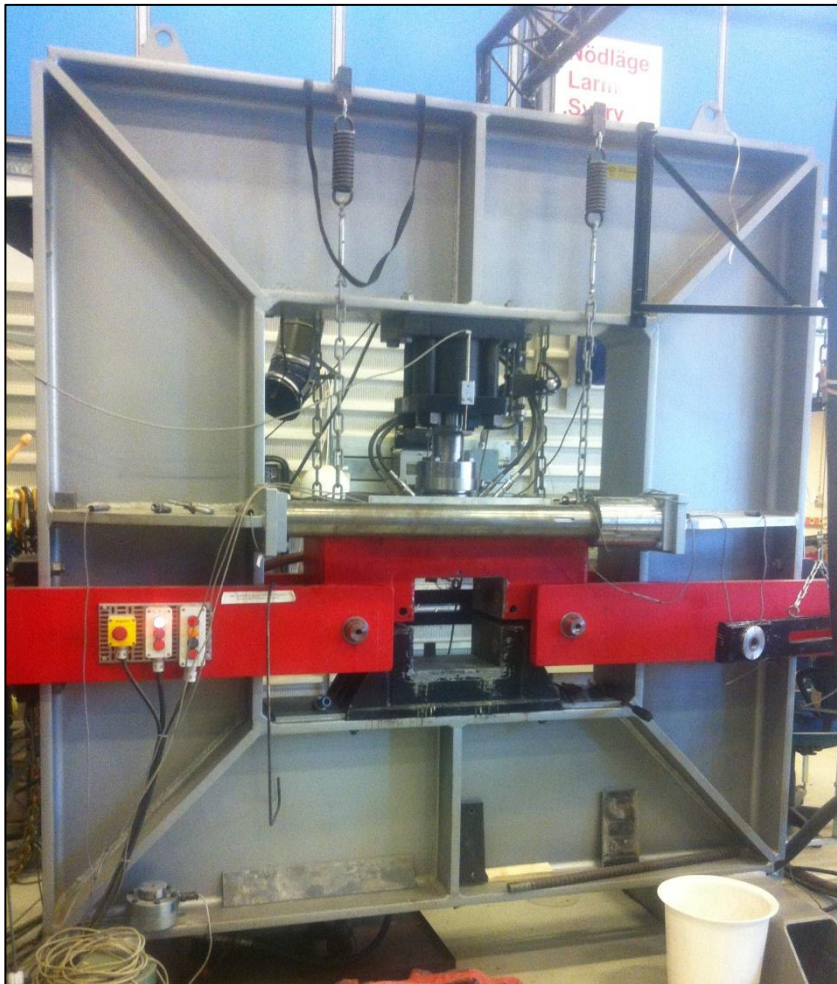
Figure 69. Direct shear test machine used in the tests at LTU.
