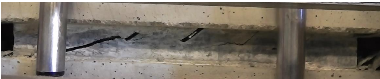
Figure 110. Test 1.2 after the bond breaking.
