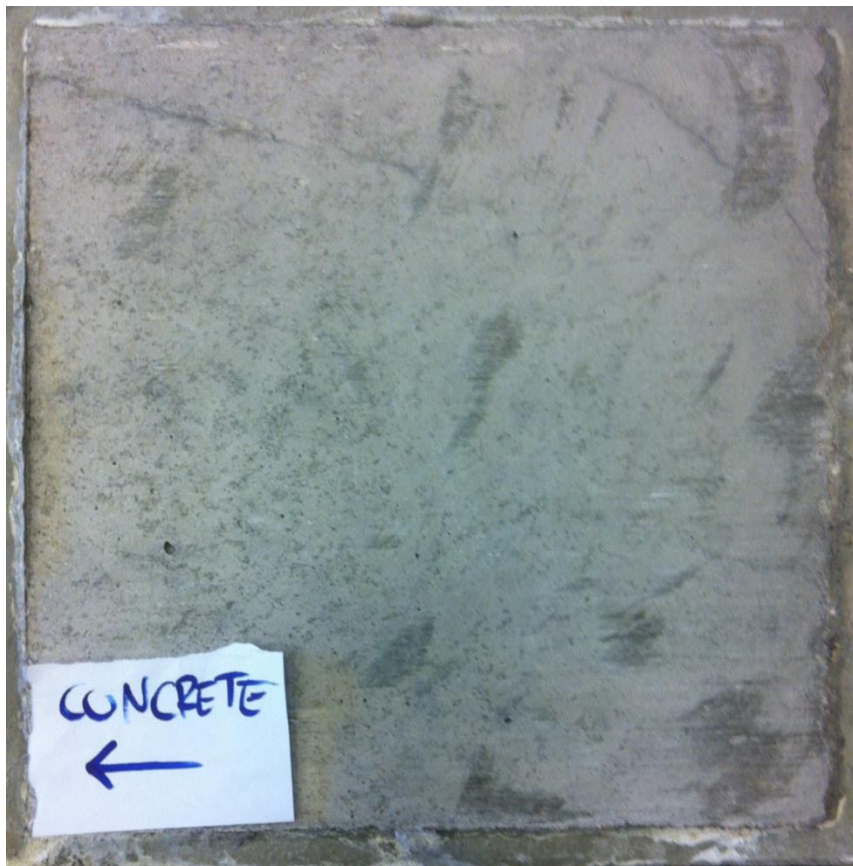
Figure 155. Test 4.1 Concrete interface after the test.
