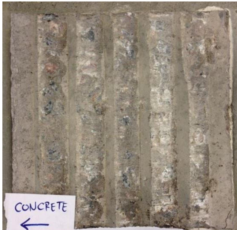
Figure 125. Test 2.1 Concrete interface after the test.
