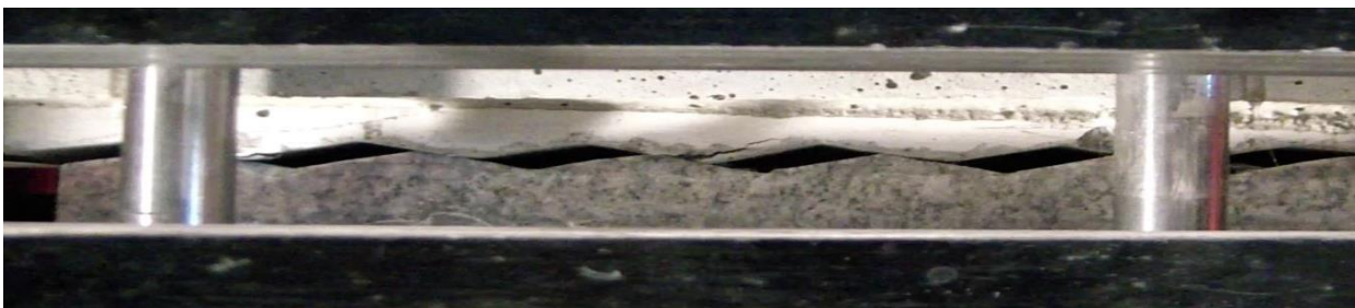
Figure 51. Test 3.1 Interface when peak shear stress is reached (taken from (Liahagen, 2012)).
