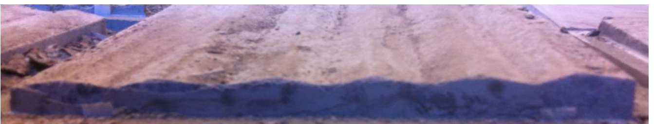
Figure 151. Test 3.3 Rock asperities after the test.
