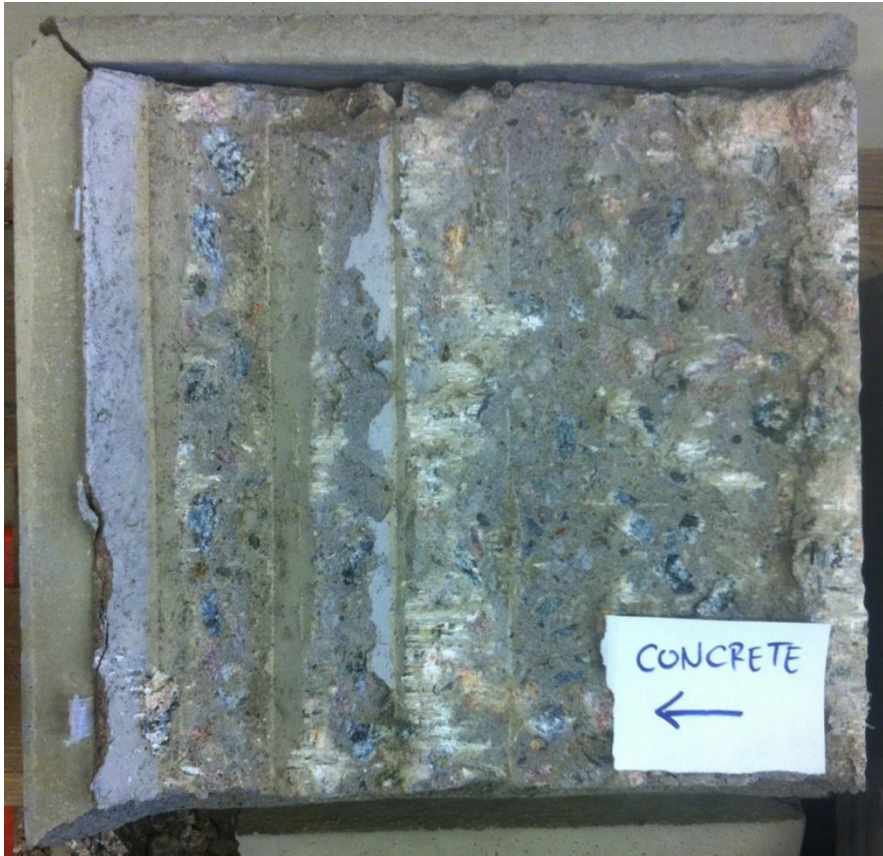
Figure 107. Test 1.2 Concrete interface after the test.
