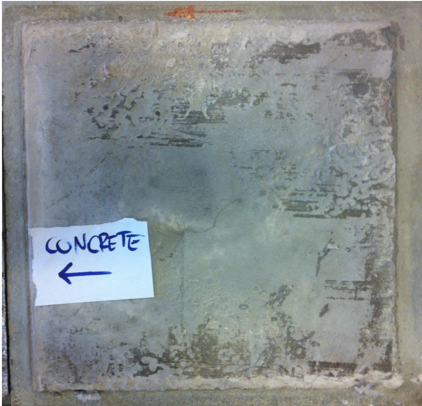
Figure 160. Test 4.2 Concrete interface after the test.
