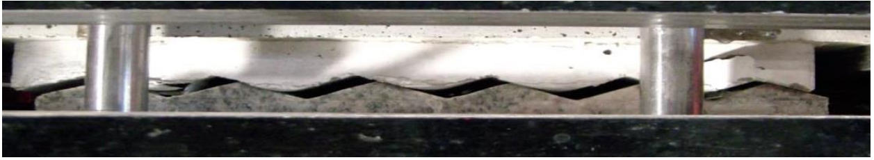
Figure 52. Test 2.1 Interface when peak shear stress is reached (taken from (Liahagen, 2012)).
