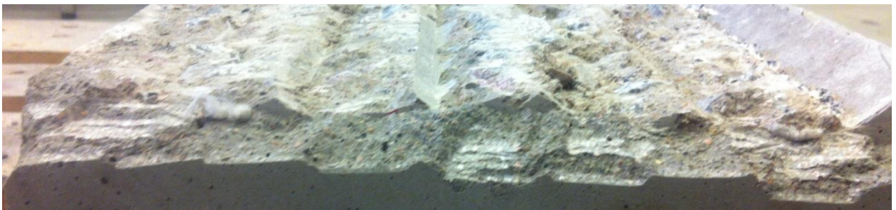
Figure 124. Test 1.4 Concrete asperities after the test.
