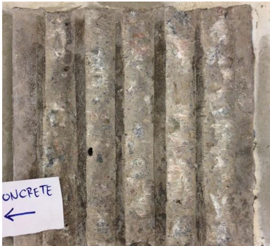
Figure 129. Test 2.2 Concrete interface after the test.
