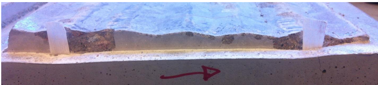
Figure 145. Test 3.2 Concrete asperities profile after the test.
