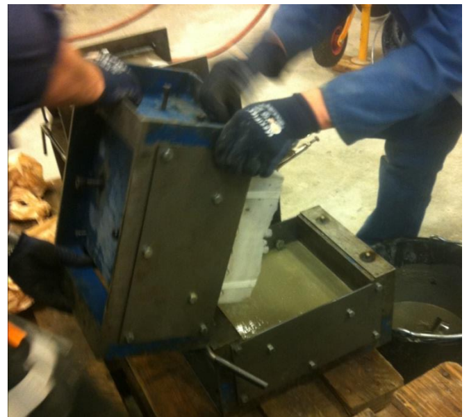
Figure 78. Casting on the steel molds (ii).
