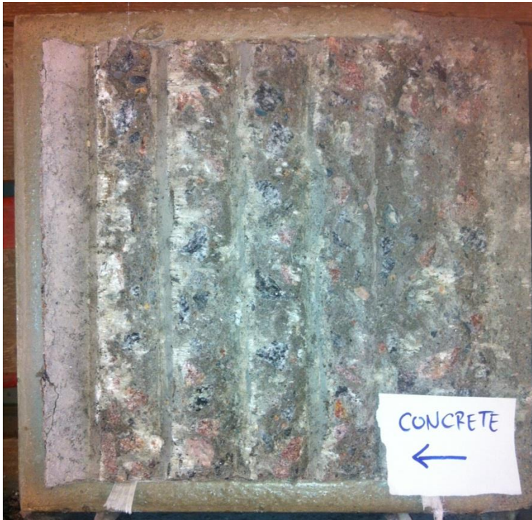
Figure 101. Test 1.1 Concrete interface after the test.
