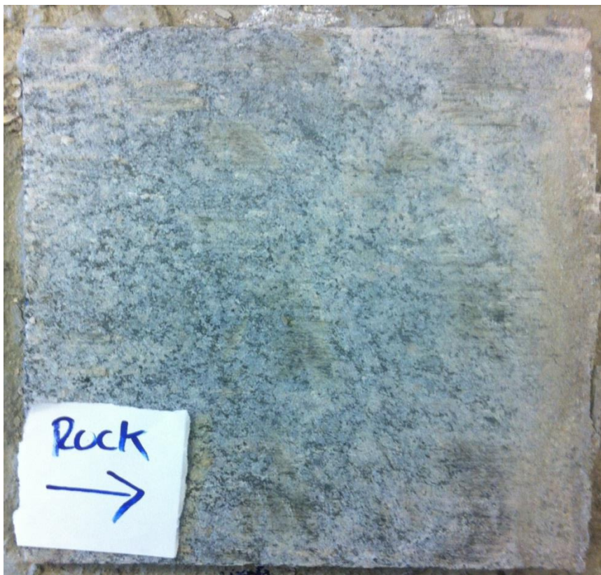
Figure 156. Test 4.1 Rock interface after the test.
