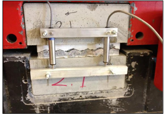
Figure 38. LVDTs glued to the specimens (taken from (Liahagen, 2012))
