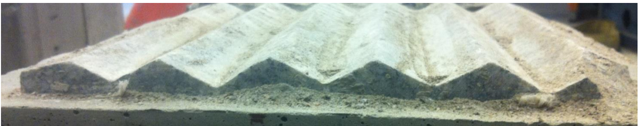
Figure 135. Test 2.3 Rock asperities profile after the test.
