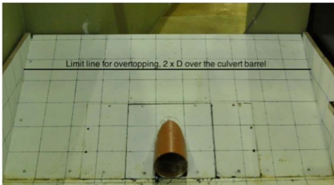
Figure 4.6 Limit for overtopping
