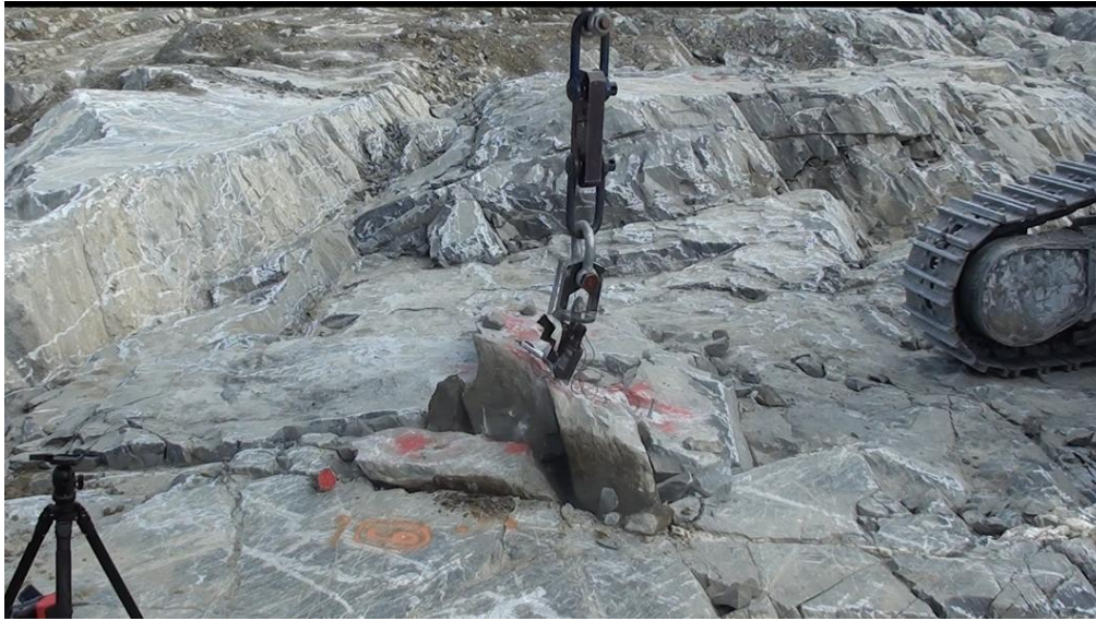
Figure 47 : Break inside the cone of influence, Verdalskalk 2012, bolt nr 3
