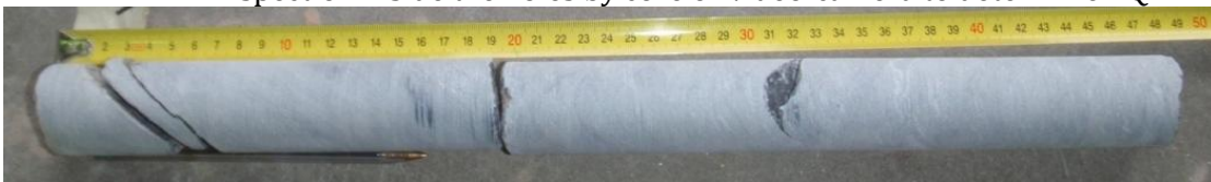
Figure 36 : drill core : some cracks are due to coring
