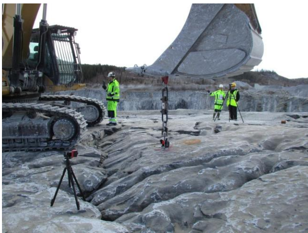
Figure 41 : 2 video cameras to record large rock behavior around bolt and strength-deformation logging devices
