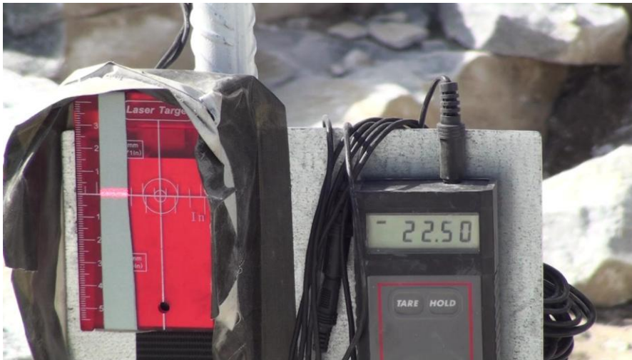
Figure 39 : System for load and deformation measurement, recorded by a video camera
