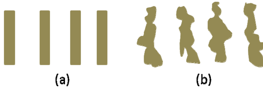
Figur 9: (a) Modelled pore structure, (b) actual pore structure (Mulder 1996).
