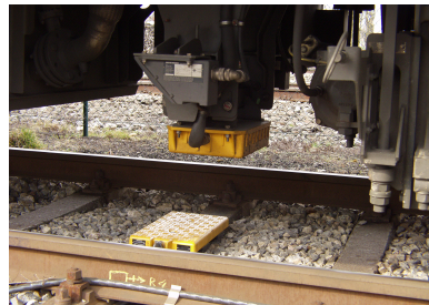
Figure 2.1: ETCS Eurobalise ground equipment and train antenna module, image from http://www.siemens.com/press/en/presspicture/
