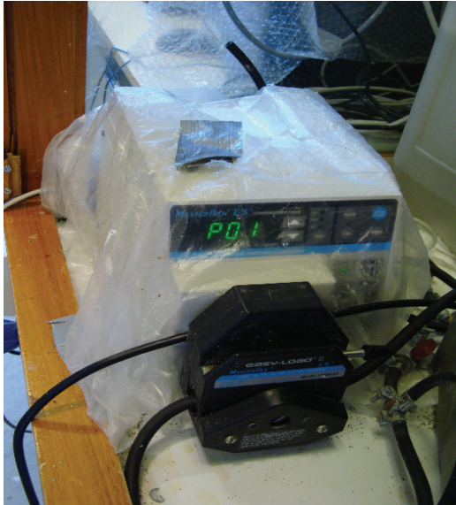
Figure 86. Peristaltic pump used to supply BTX, acetic acid and nutrients solution in the FBR
