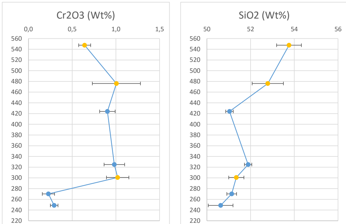
Figure 4.43 EPMA analysis showing the Cr 2 O 3 content and SiO 2 content in clinopyroxene. Points marked by yellow colour is analysed by one grain, therefore have low statistical significance
