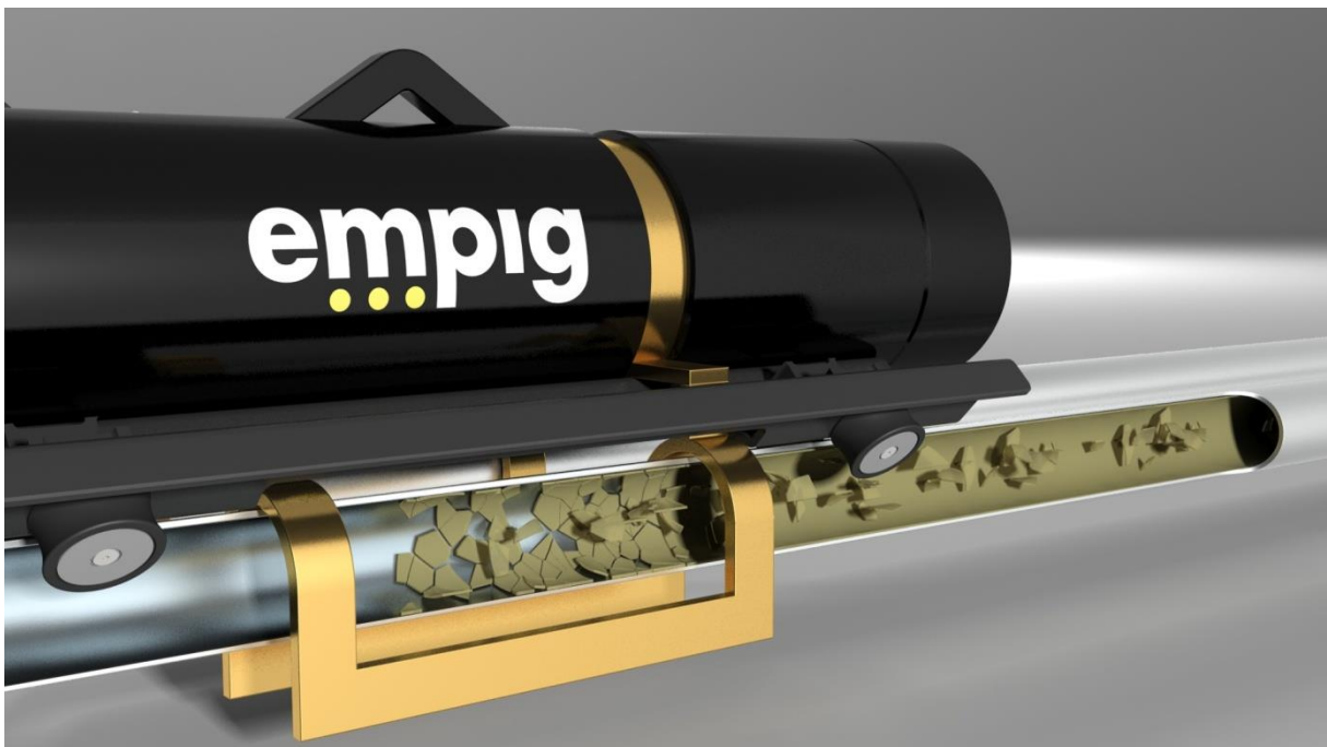
Figure 5-7 - EMPIG Inflow wax removal concept, propulsion system
