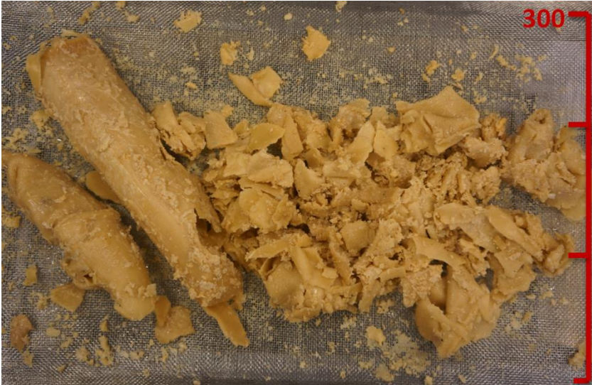
Figure 4-43 - Removed wax from pipe. Test 2.2: Downstream coil movement, 15 kW output power.
