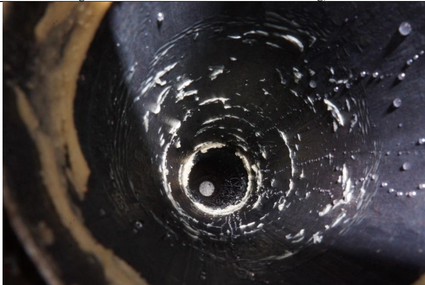
Figure 4-51 - Pipe after wax removal (looking downstream). Test 5: Scan heating, 6 kW
