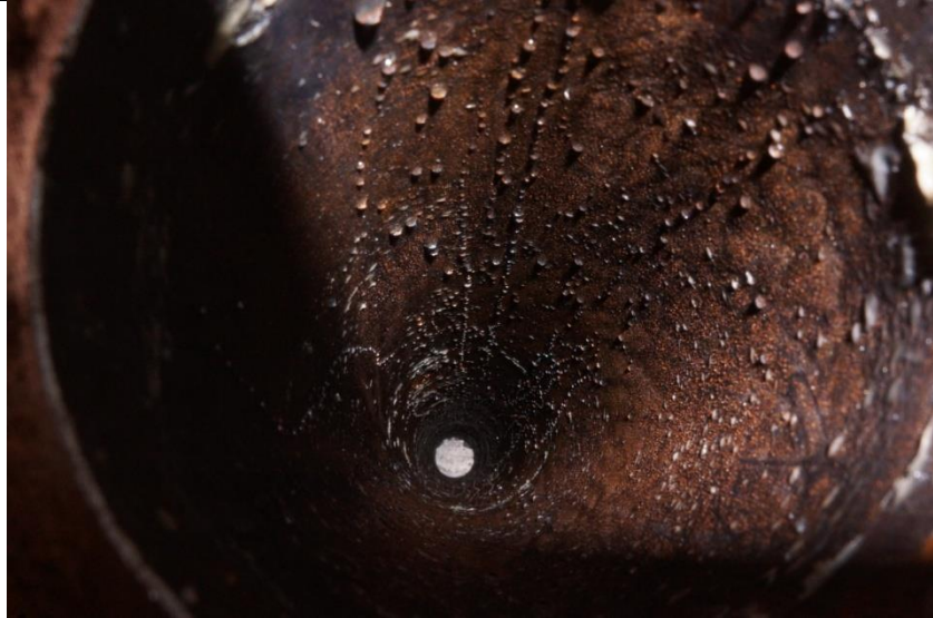
Pipe after wax removal (looking upstream):
