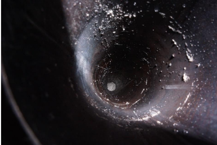
Pipe after wax removal (looking upstream):
