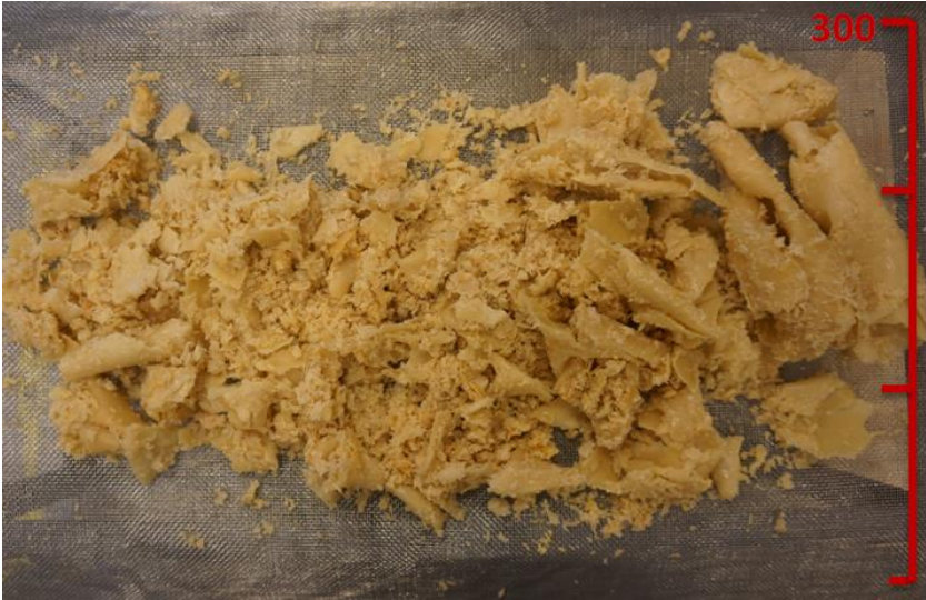
Figure 4-42 - Removed wax from pipe. Test 1.2: Upstream coil movement, 15 kW output power.
