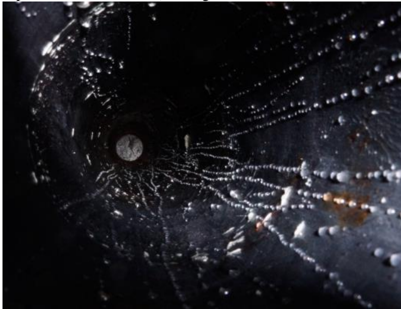
Pipe after wax removal (looking upstream):
