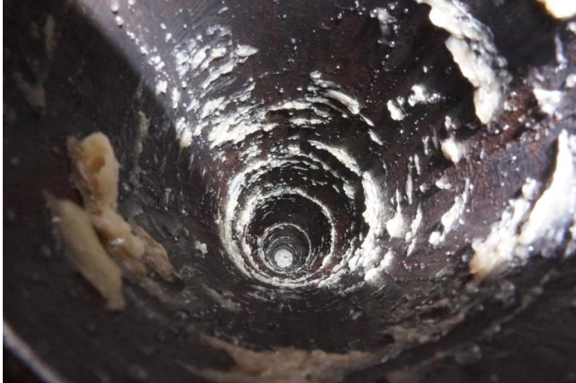
Pipe after wax removal (looking upstream):
