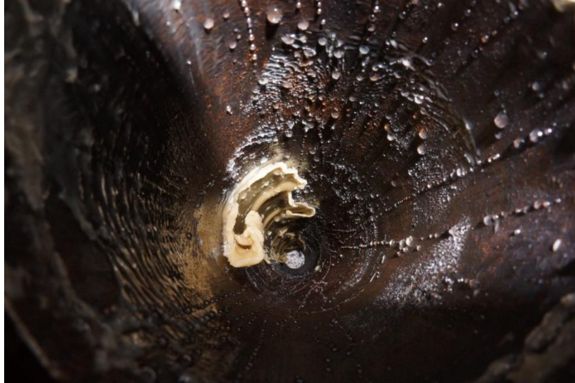
Pipe after wax removal (looking upstream):
