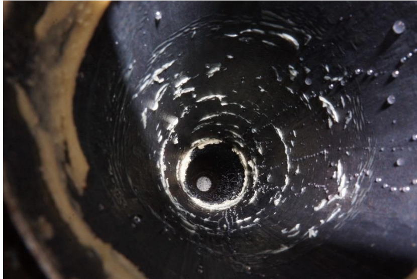
Pipe after wax removal (looking upstream):
