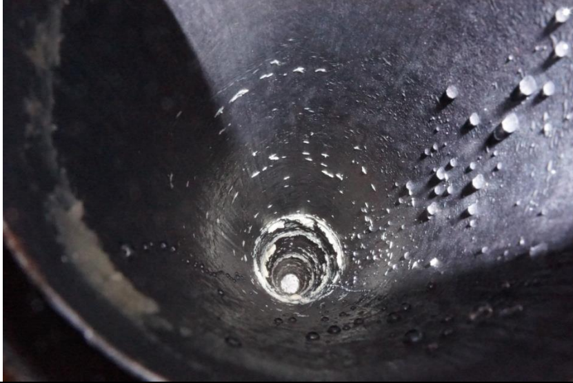
Pipe after wax removal (looking upstream):
