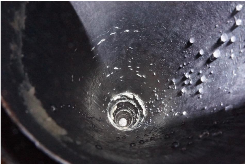
Figure 4-44 - Inside of pipe after wax removal. Test 1.2: Upstream coil movement, 15 kW output power.
