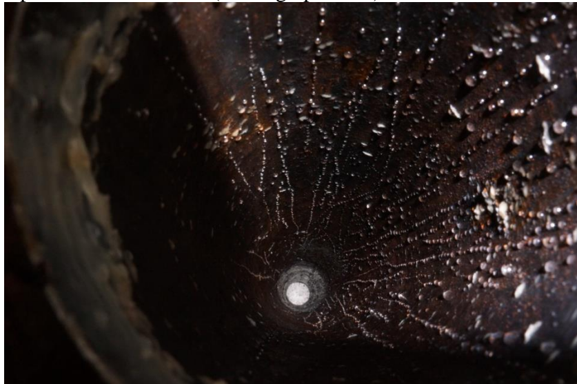
Pipe after wax removal (looking upstream):
