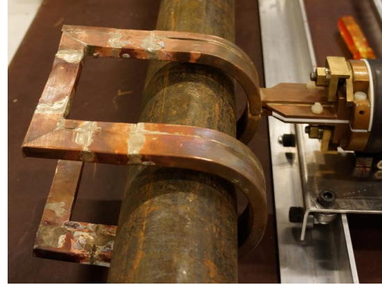
Figure 4-13 - Retrievable induction coil - Mounted in linear actuator system and positioned over pipe
