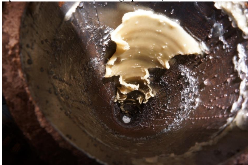
Pipe after wax removal (looking upstream):
