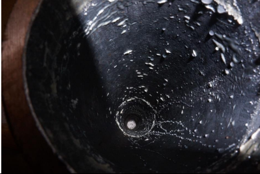
Pipe after wax removal (looking upstream):
