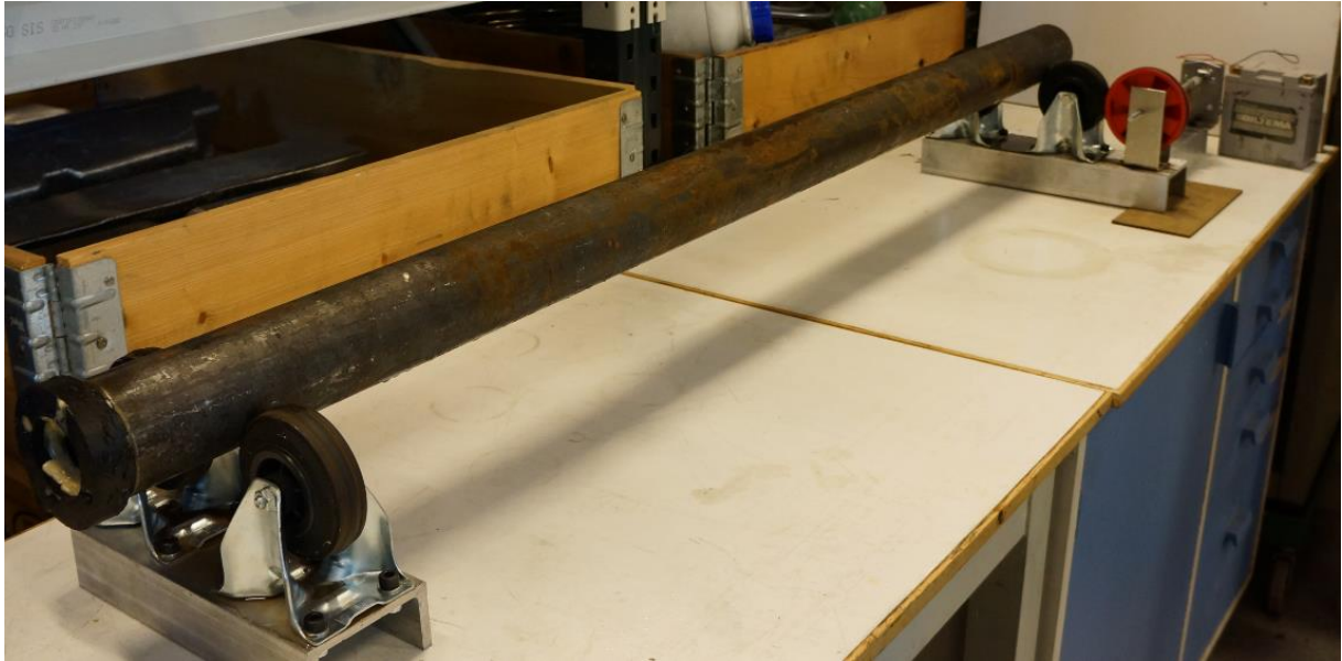
Figure 4-8 - Wax applying setup - Steel pipe positioned
