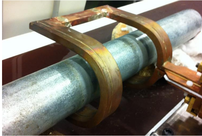
Figure 4-31 - Galvanized pipe positioned in induction coil
