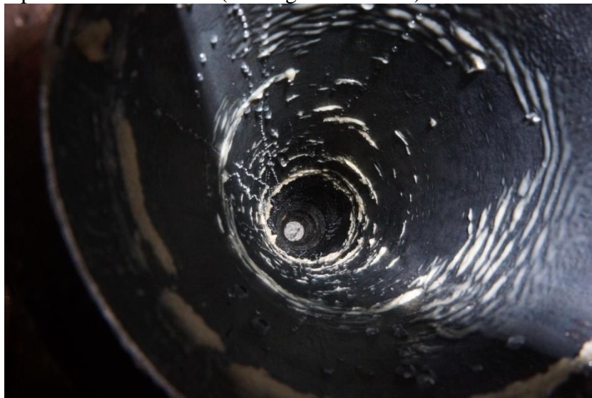
Pipe after wax removal (looking upstream):
