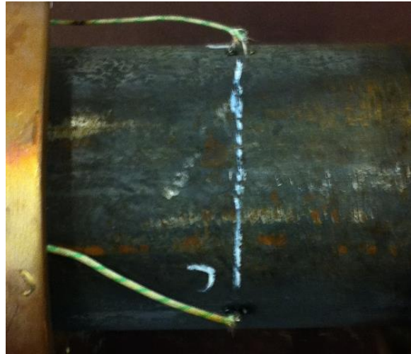
Figure 4-24 - Type-K thermocouples welded to pipe surface
