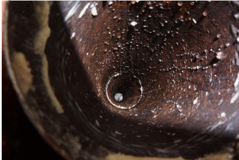
Pipe after wax removal (looking upstream):
