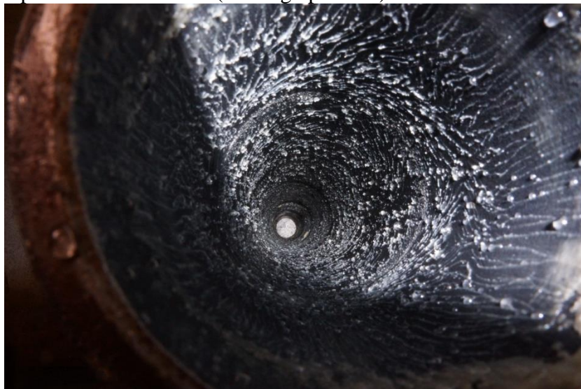
Pipe after wax removal (looking upstream):
