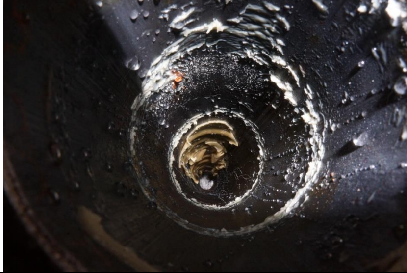
Pipe after wax removal (looking upstream):
