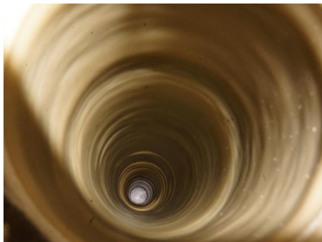
Figure 4-21 - Wax applied on steel pipe inner wall
