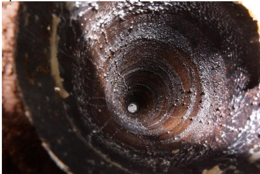
Pipe after wax removal (looking upstream):
