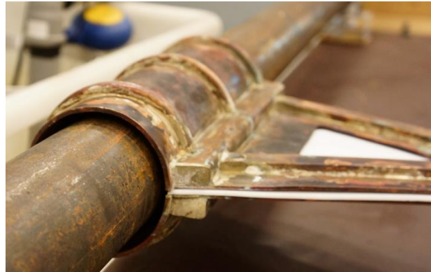
Figure 4-17 - Non-retrievable induction coil - Mounted in linear actuator system and positioned over pipe
