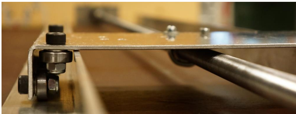
Figure 4-7 - Linear actuator – sleigh held in place by bearings and guiding rails
