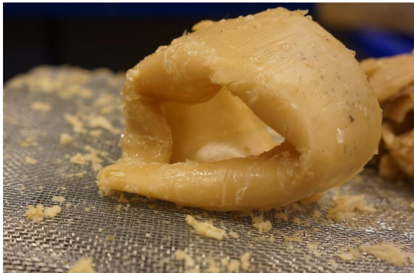
Figure 4-46 - Close up of wax debris from Test 2.1: 10 kW power, coil moving downstream.
