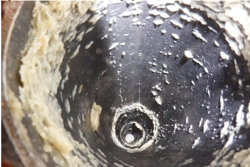
Pipe after wax removal (looking upstream):
