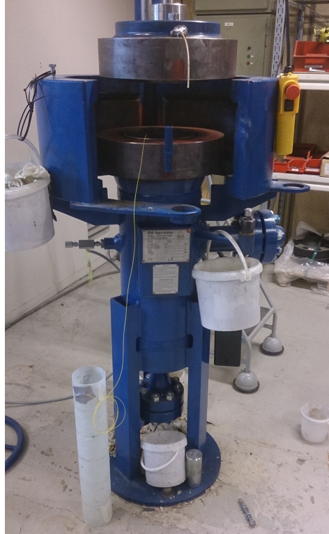
Figure 4.1: Autoclave and tube without endcaps, with the signal wire escaping the autoclave through the T-fitting seen on the left side of the autoclave.
