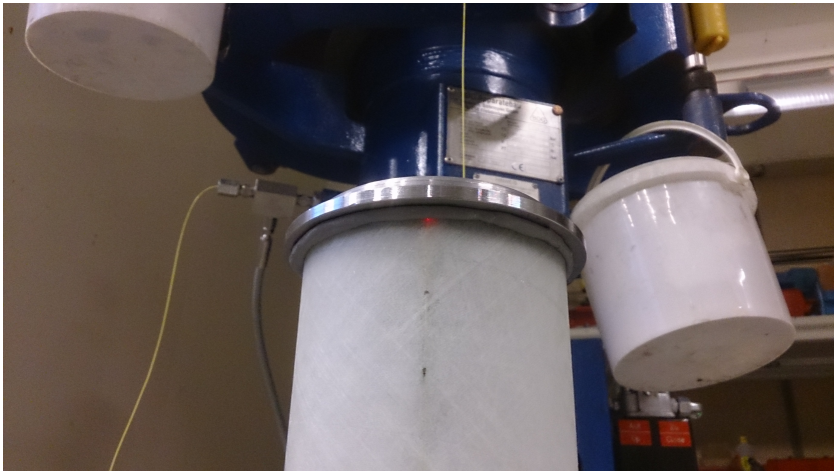
Figure 4.3: Endcap applied with stickytape. Also visible in the background is the T-fitting.
