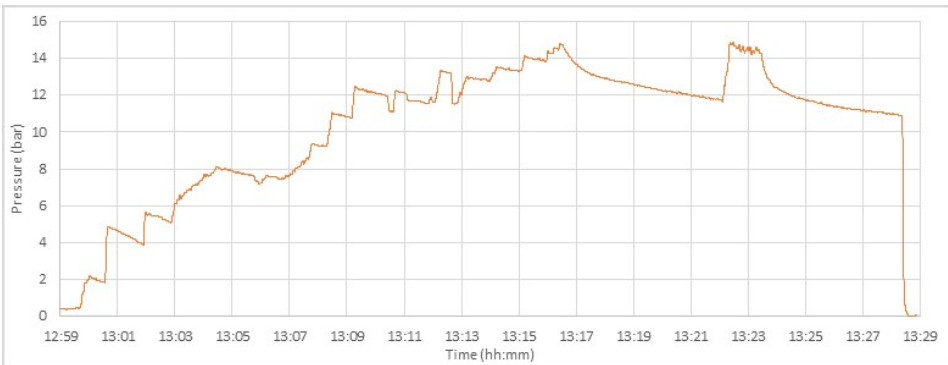
Figure B.17: Pressure reading from test nr. 2 of the 400 mm long tube, smoothed using Matlab.
