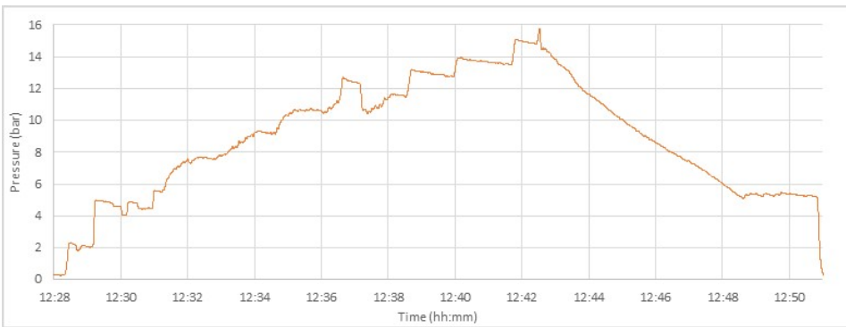
Figure B.15: Pressure reading from test nr. 1 of the 400 mm long tube, smoothed using Matlab.
