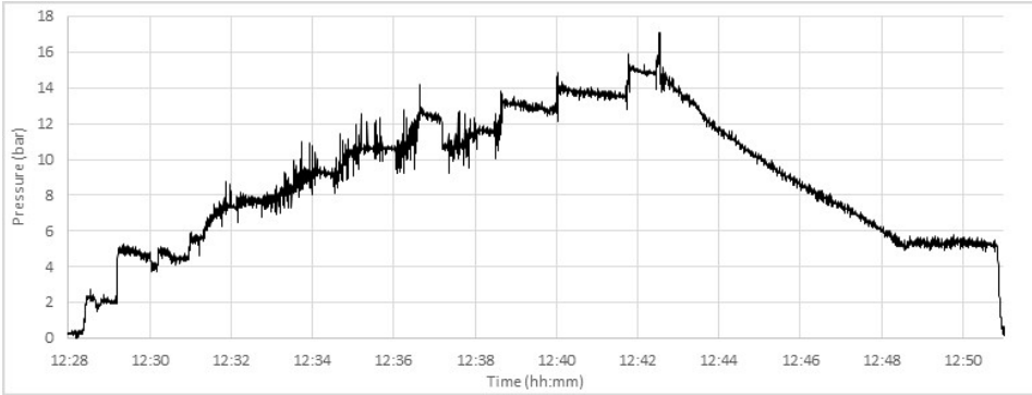
Figure B.14: Pressure reading from test nr. 1 of the 400 mm long tube.
