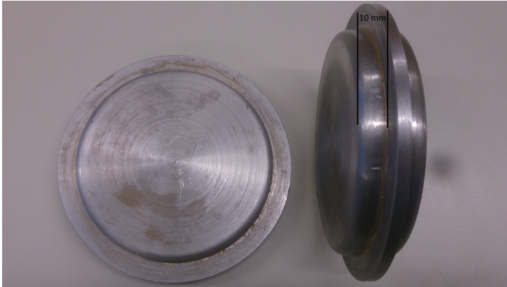
Figure 4.2: The two endcaps used for sealing the ends of the tube. Also shown is the stick out of 10 mm.
