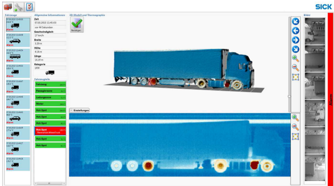
Figure 2.7: Example of 3D image with thermal results obtained from the thermal portal
