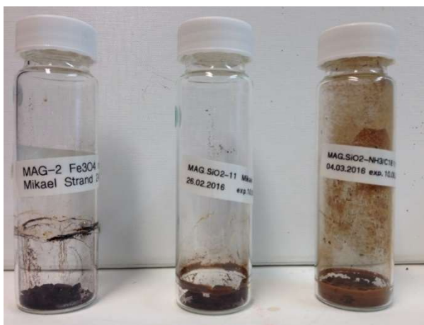
Figure 6.7: Dried magnetic nanoparticles, from left to right: \text{Fe}_3\text{O}_4 -1.1, \text{Fe}_3\text{O}_4/\text{SiO}_2 -1.1 and \text{Fe}_3\text{O}_4/\text{SiO}_2 \text{NH}_2/\text{C}_{18} -1.1.1-t.
