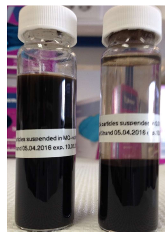
Figure 6.5: Fe_3O_4 naked magnetic nanoparticles in Milli-Q water (left flask) and in a solution of HCl (right flask).
