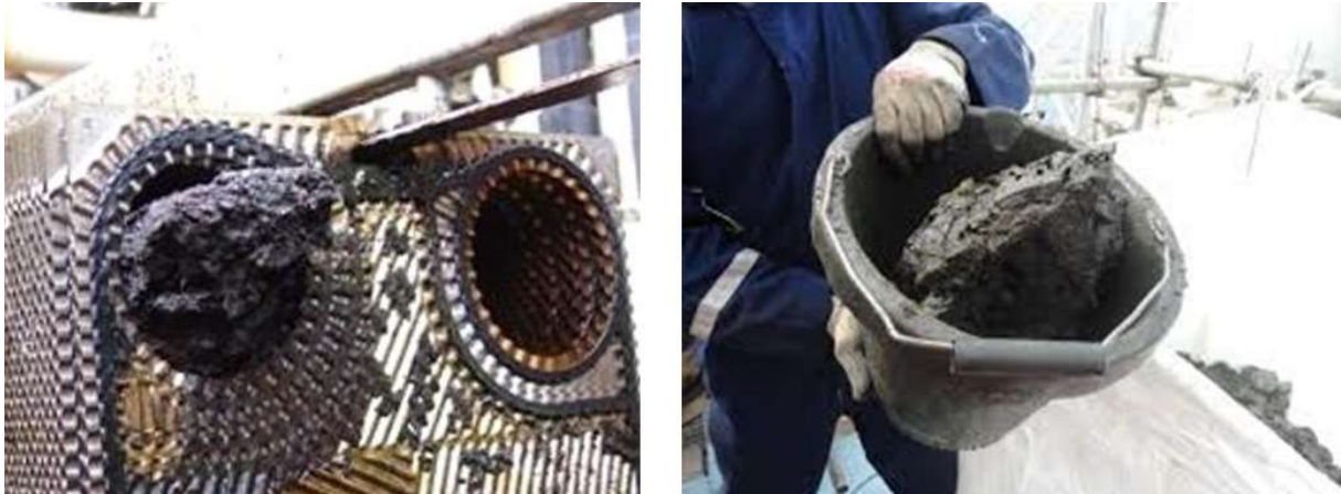
Figure 1.3: Naphthenate deposits in a cooler [10] and deposits removed from a coalescer [11].
