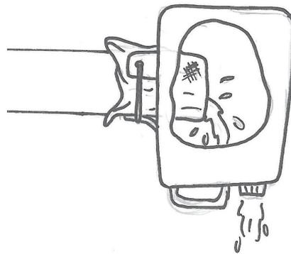
Figure 53 Filter on end of gutter
