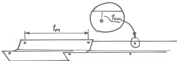
3. Starting at the opposite end of where the drop outlet will be, thread the wire through the gutter hole closest to the wall, and tighten.
