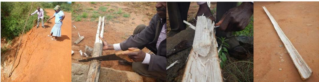
Figure 32 Sisal gutter - image sequence
