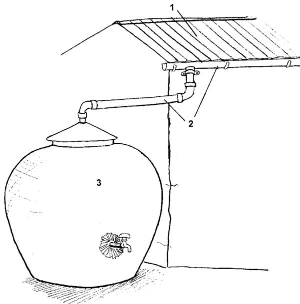
Figure 16 Roof top catchment, basic principles. Source: Worm and Hattum (2006)
