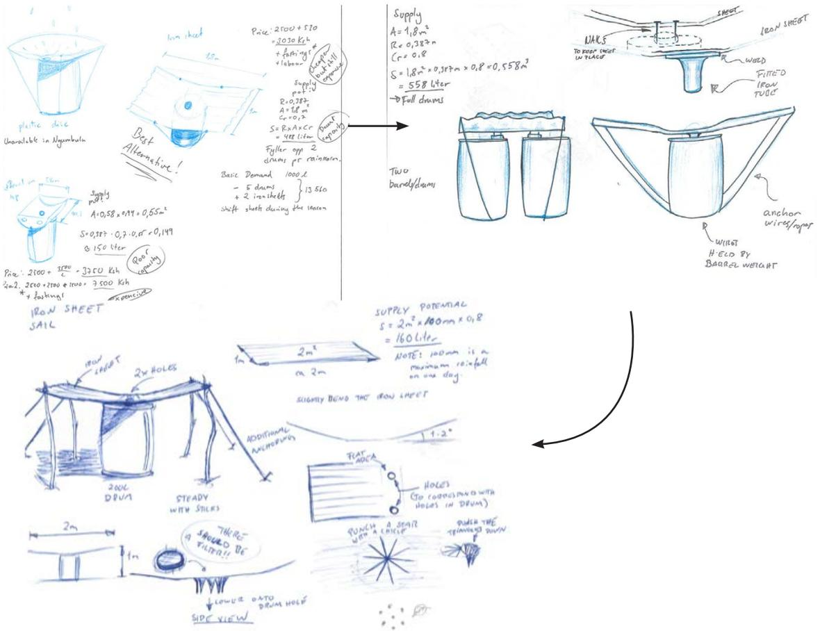
The concept has the advantage of being stable and efficient even in strong winds and is not required to be uninstalled between each rain. During the heat the iron sheet provides shadow and protection for the reservoir. Issues lies in the capacity per system as a maximum of 3m<sup>2</sup> of catchment surface is possible and the reservoir is somewhat small.
