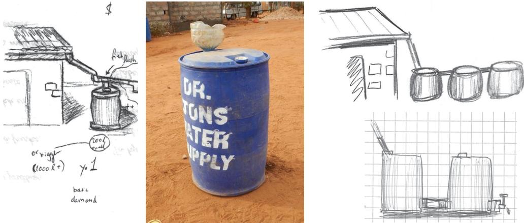
The tanks leave no possibility of local production and must be imported from Katangi. The drums are lightweight and may be used to transport water from the river when empty from rainwater. Drums have a capacity issue and are somewhat expensive per liter, but introduction cost is low and incremental increase of storage is easy.
