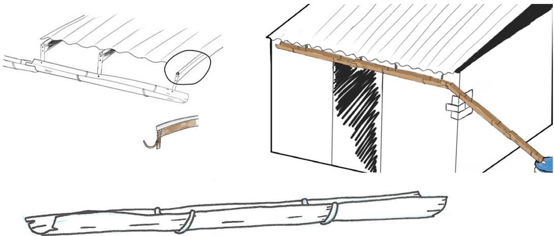
The discussion revealed that even though the sisal seems good for gutters; it may not be possible as a drop outlet. There will be severe issues in fastening of this, as well as a long stem is required. Also the need for extra support of this render the concept difficult to make and the durability is questionable.
