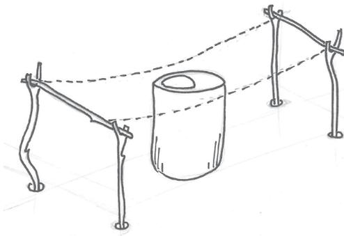
7. While the iron sheet is resting on both pole frames and the drum, check that there is a slope on both sides towards the middle. Adjust the hole depth if needed.
