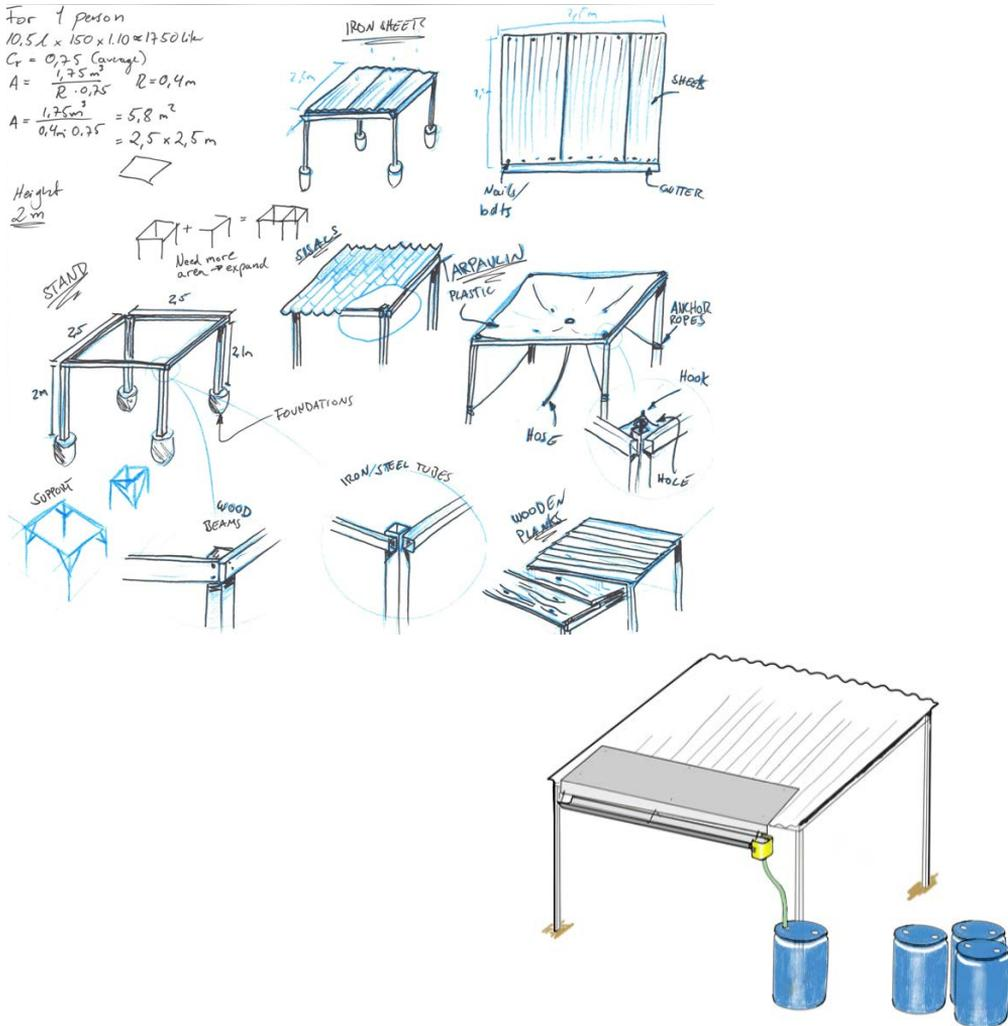
The idea is to simulate a house by constructing a framework of timber overlaid with iron sheets. In addition gutters and a reservoir is needed in the same way for a rainwater harvesting system installed on a regular house. This implies great costs and may not be suitable for the most economically challenged in the community, however may serve as an addition for those with iron sheet roofs.
