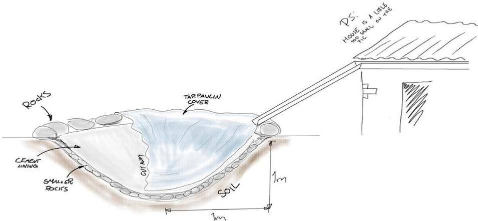
The walls must perhaps be cemented or plastered with rocks to prevent erosion of the walls, which will add cost. There may also be a safety issue with retrieving water, as the walls need to be sloped. Also the large surface area gives a cover problem, and by not having a covered tank, mosquitoes may present a disease issue by breeding in the reservoir.
