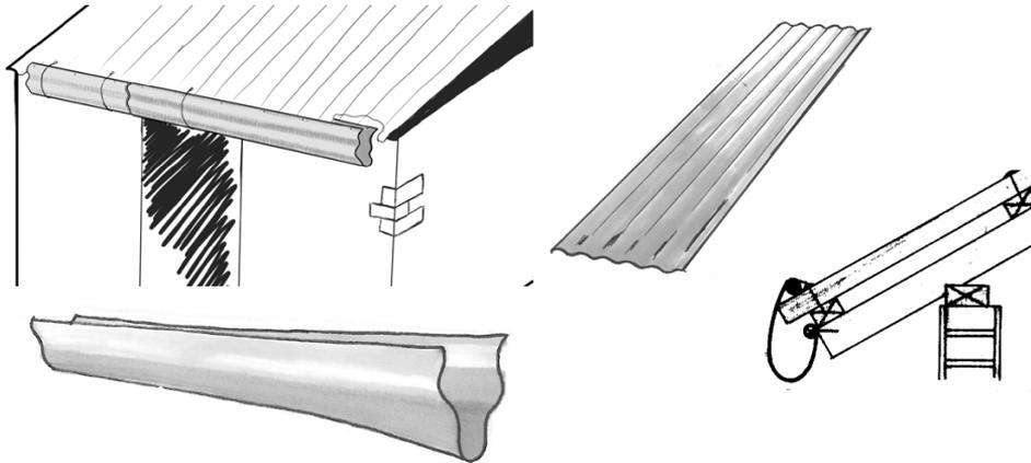
This type has been seen in Ngumbulu and is known by the community. It is simple to make, durable and efficient. However it is not cheap as a rather wide part of the iron sheet must be used, and the closed fashion of the gutter makes it hard to keep clean. There is also an issue with the drop outlet, but a jerry can seems to be a solution for this.
