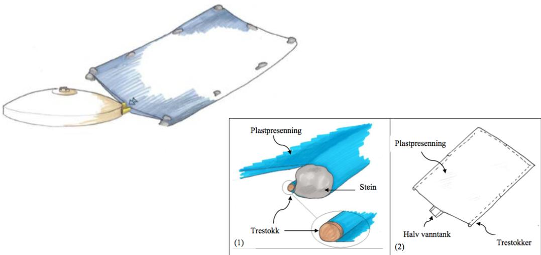
an underground concrete tank. The concept is dependent on a flat surface without vegetation angled towards the tank. After each rain the tarp is to be rolled up and stowed away waiting for the next pour.
