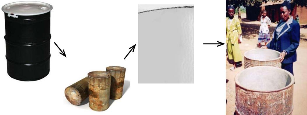
This tank is potentially very cheap and may be produced locally because of the easy construction. The durability becomes very high, and it may even be somewhat mobile. Drums can usually contain 200 liters incremental increase of storage is easy
