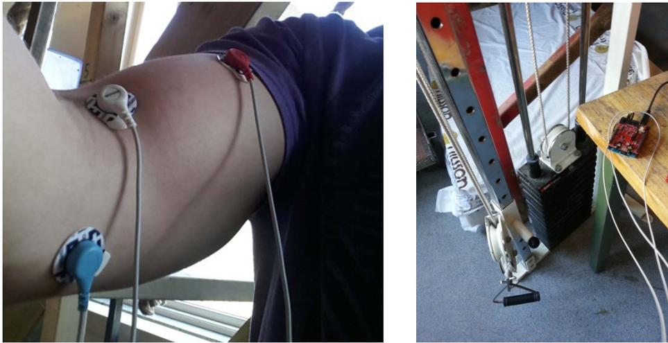
Unfortunately there was not taken any pictures of the other attachment to compare, but this is the attachment from the first test day which was used on *first test* in table 5. The middle electrode is here placed high up on the arm, making the electrode to be on center of the biceps when fully flexed. If the electrode was attached more on the center of the upper arm when stretched out, the electrode will “fall off” the biceps when flexing.
