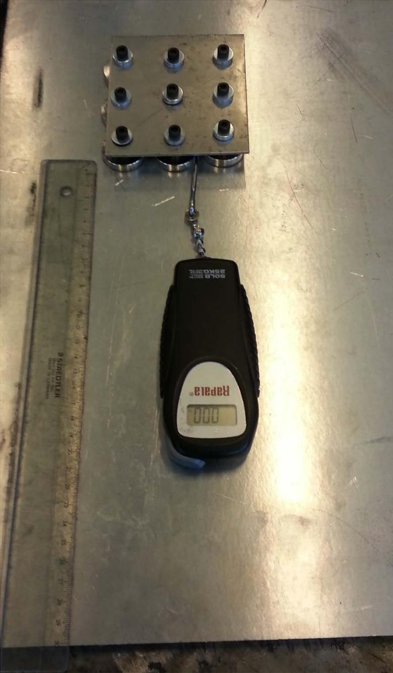
The same test was done on a welding table of steel to see what kind of force the magnets would generate against a steel plate. This is not eddy current working and the force will therefore not be affected by speed.
