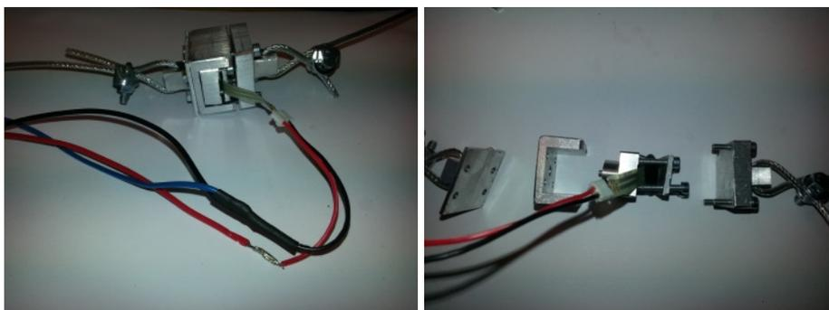
**Figure 15: Homemade load cell, exploded view to the right (see appendix H)**
