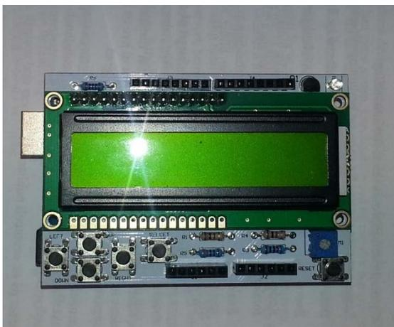
**Figure 16: The LCD breakout board**
