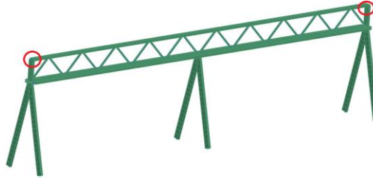
Figure 6-12: Location of Vertical Profile–Top Beam 90° Connections (marked in red)
