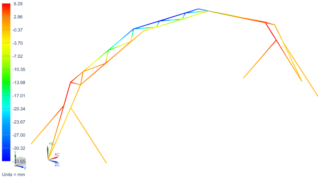
Figure 4-26: Model II – 20m: Vertical Displacement Results
