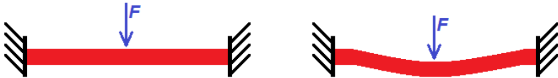
Figure 2-5: Behaviour of a beam fully fixed in both ends subjected to a vertical load
