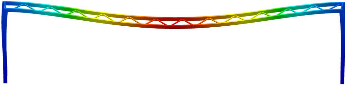
Figure All-5: Behaviour of the Boom's deflections in a Gantry
