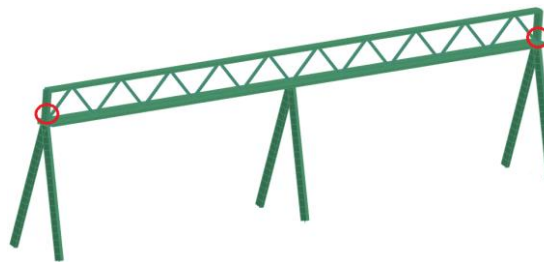
Figure 6-15: Location of Vertical Profile–Bottom Beams 90° Connections (marked in red)
