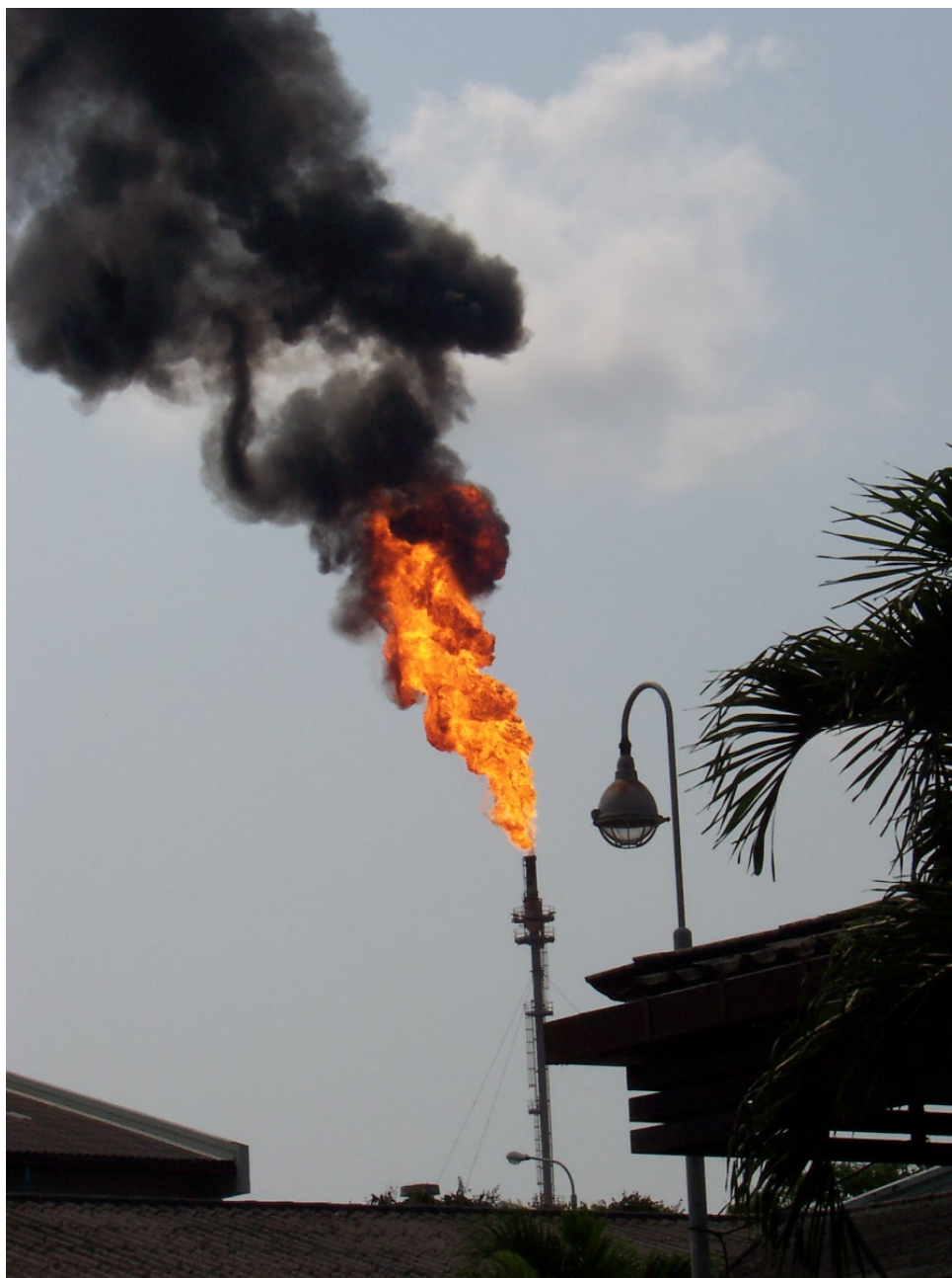
Figure 1.1: Photo of a gas flare in Thailand. The photo is taken from Krittaya (2007). Notice how the BC form a seemingly black smoke due to the very high concentration of BC released in the plume.
