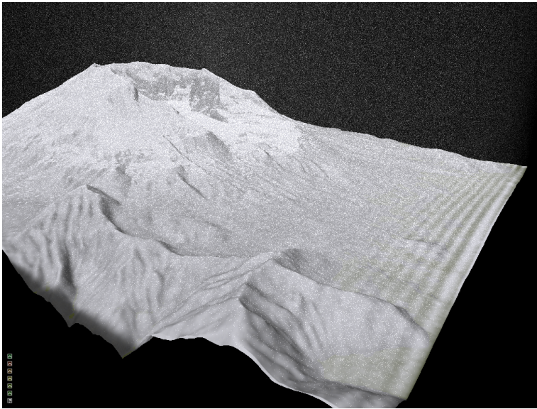
Figure 3.6: A visible pattern in accumulated snow due to stability problems in the SOR solver.
