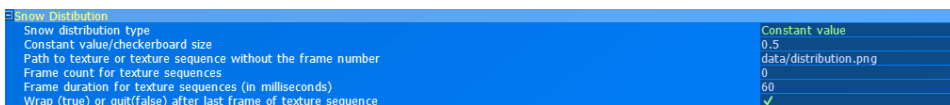
Figure I.4: All precipitation distribution settings. If the Constant value strategy is used, only the two first entries have meaning.
