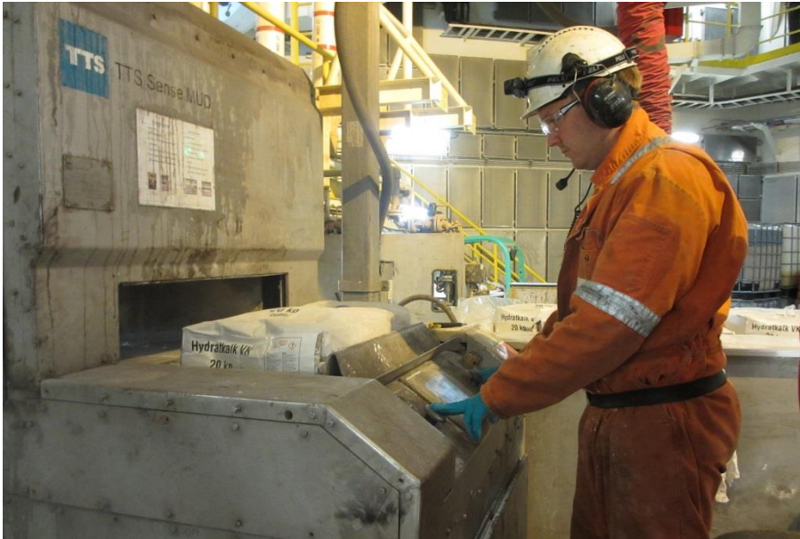
Figure 9 - Adding powdered chemicals using the SDU (photo: Sondre Buset Bjelland)
