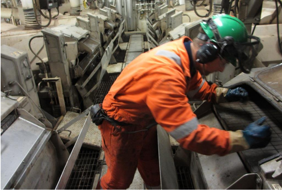
Figure 24 - Brute force required to attach the screen (photo: Sondre Buset Bjelland)
