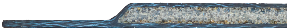
(A) Cross section of Tc2, the foam is the core material which adequately fills the gap between the lower and upper skin.
