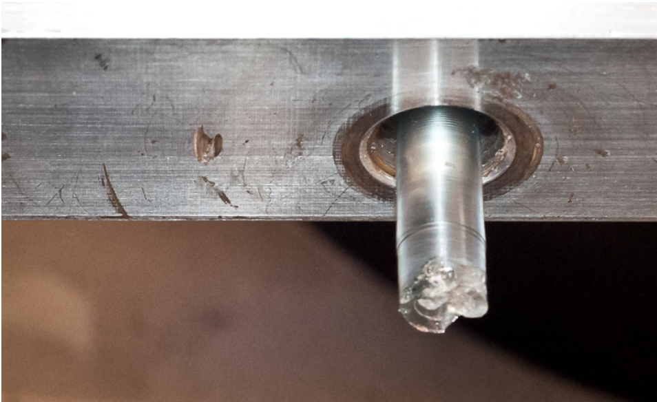
FIGURE 7.7: The picture shows resin cured in the tool sprue.
