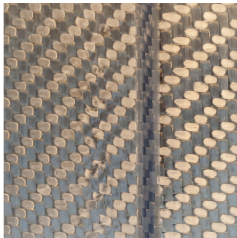
(C) The transition to the core material in Tc2. No visible surface flaws.
