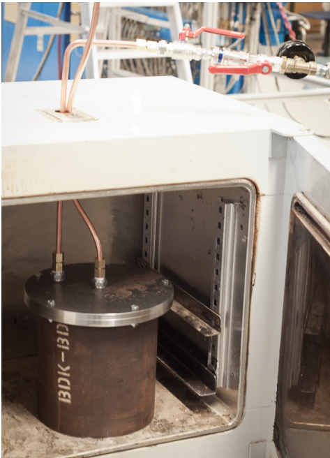
(A) The resin pressure pot in side an oven as it was used in the experiments.
