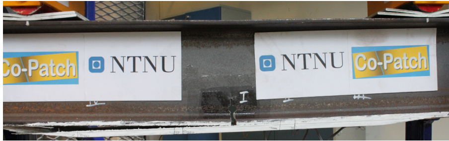
Figure 78: After failure, beam 36.
