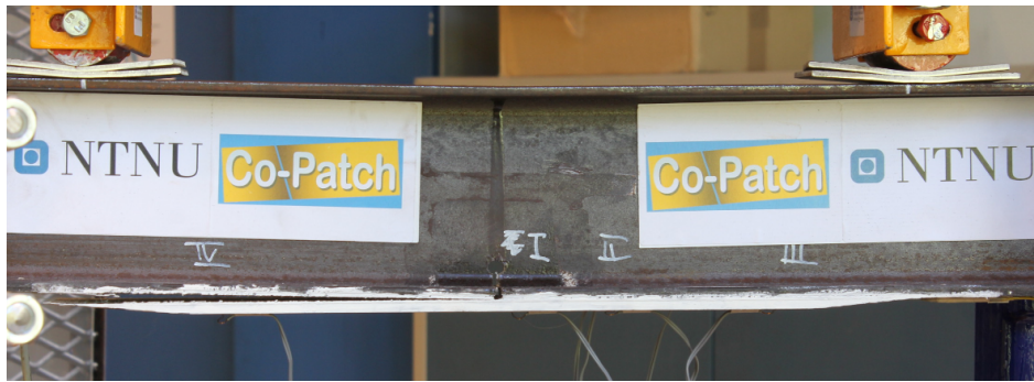
Figure 58: Beam 32 after failure. Debond and cohesive failure on the left side.
