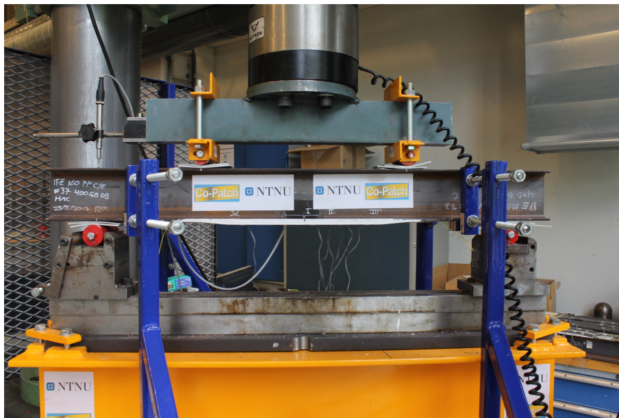
Figure 27: Actual setup of the four point bend test at IPM NTNU.
