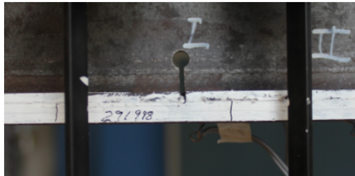
Figure 46: Damage propagation from center towards both ends. Front of beam 21.
