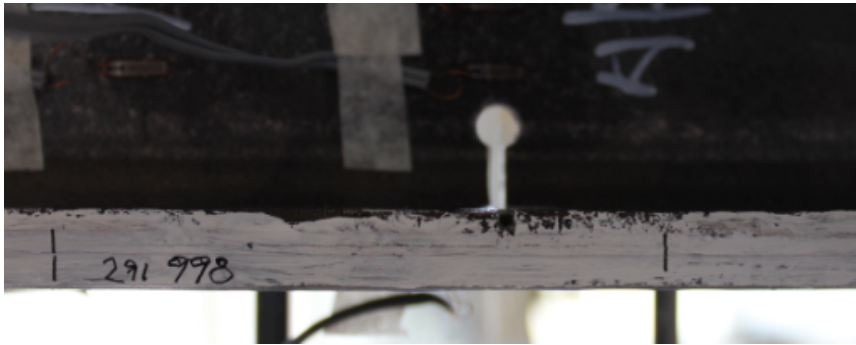
Figure 47: Damage propagation from center towards both ends. Back of beam 21.
