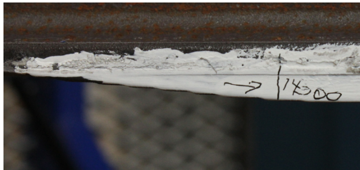
Figure 77: Damage propagation from left at 14 700 cycles. Beam 36.
