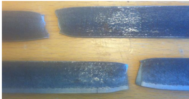
Figure 3-2: Rupture of specimen 4.2 (top) and 4.3 (bottom).
