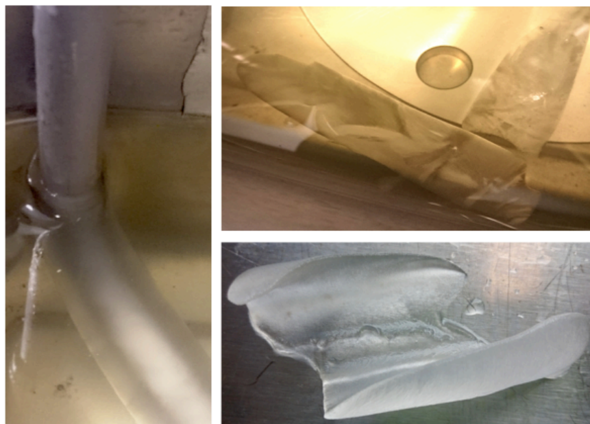
Figure 3.1: Hydrate deposit on the steel pipe (left) and after removal from the pipe (right). The upper right picture shows the hydrate while floating in the tank fluid, in the lower picture it is placed on a dry surface at room temperature
