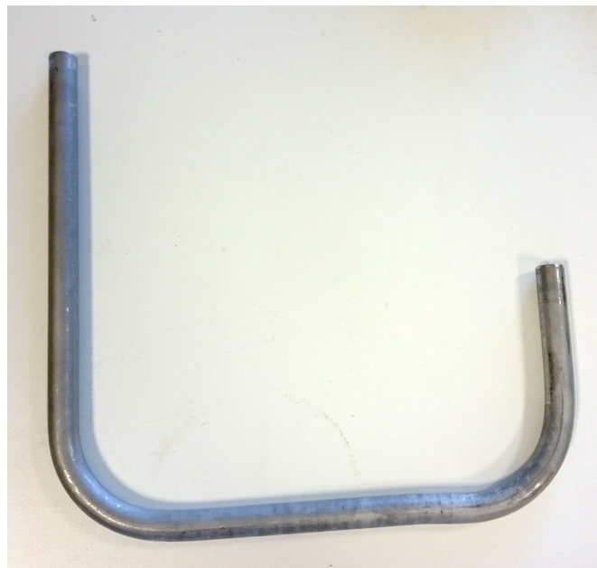
Figure 2.2: The steel pipe with high roughness. The section to the right is where the scraping was conducted
