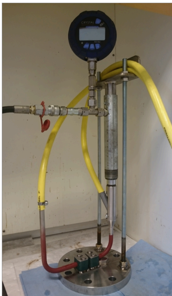
Figure 2.5: Picture showing the steel pipe attached to the flange with holders and to the scraping mechanism. The yellow hoses are connecting the pipe and the cooler, while the black hose to the left is connecting the pump to the piston. The manometer is at the top
