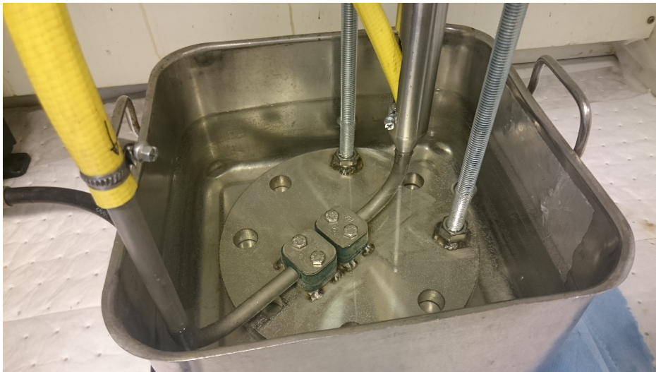
Figure 2.6: Picture showing the pipe submerged in the tank filled with THF and water. The scraper is seen to the right between the two rods
