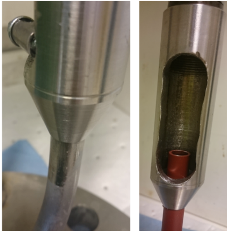
Figure 2.3: Pictures showing the cylinder for scraping. To the left is a close-up of the angled section of the cylinder and the pipe inside. The picture to the right shows the slit made to attach the pipe (red) to the cooler hose (not shown)
