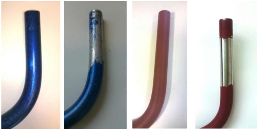
Figure 2.9: The pipe with high roughness coated with automotive paint (left) and the smoother pipe coated with corrosion-avoiding primer (right). The left pictures of each coating are before the experiments, the right ones are after
