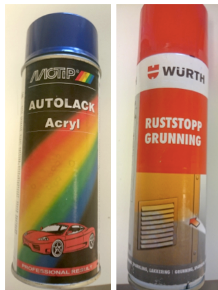
Figure 2.8: The two coatings tested in the experiments. Automotive paint on the left and corrosion-avoiding primer on the right
