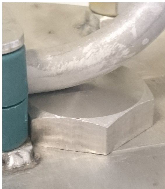
Figure 2.7: A slice of steel was placed between the steel pipe and the flange to avoid bending of the pipe
