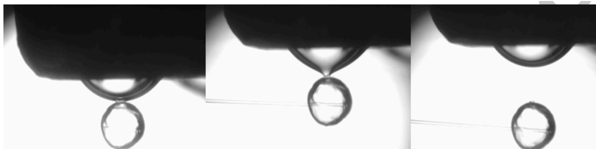
Figure 1.17: Water droplet (top) deposited on a solid surface and a hydrate particle (bottom) with acid adsorption. The liquid bridging between the two particles is very small (Aspenes et al., 2010)
