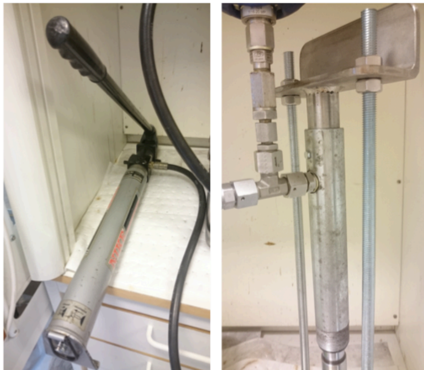
Figure 2.4: The pump (left picture) used to provide pressure to the piston (right picture). The picture to the right also shows the two rods used as holders for the piston/ scraper mechanism (seen at the bottom) and the manometer seen in the upper left corner
