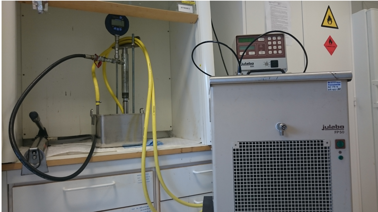
Figure 2.1: Picture showing the whole equipment setup. The cooler is seen on the right, the pump is on the left, while the pipe with the scraping mechanism is in the middle, submerged in the tank with THF and water
