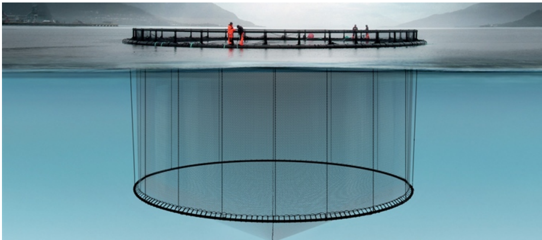
FIGURE 4.2: Illustration of a net cage. The top ring on the surface is called a floating collar, the horizontal submerged ring is called bottom rope and the vertical ropes in between, holding the mesh, are called vertical ropes [80].
