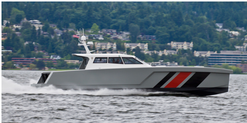
FIGURE 3.3: 57feet, long range prototype boat (LRV-17), made of carbon fiber/CNT composite by Zyvex Marine [61].
