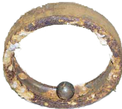
FIGURE 4.5: Photograph of roller bearing subject to water damage [92].
