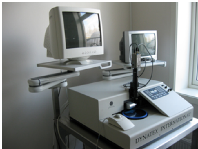
FIGURE D.1: Photograph of Dynatex DXIII Scriber [121].
