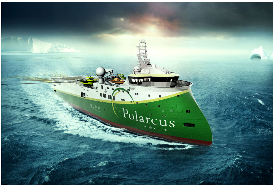
FIGURE 3.8: Illustration of a Polarcus research vessel designed for operations in arctic waters, made by Ulstein Group [69]. The bow, known as X-BOW, is supposedly inspired by Viking longships [70].
