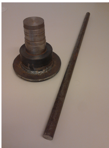
Figure 1.4: Sample of welded bushing connection and sample rod.
