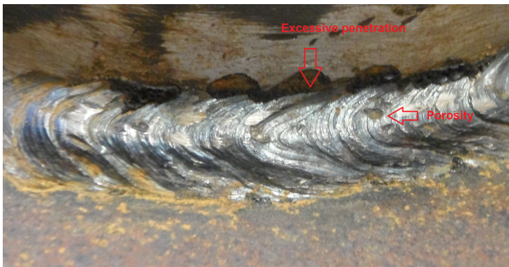
Figure 3.1: Weld on bushing and disk
