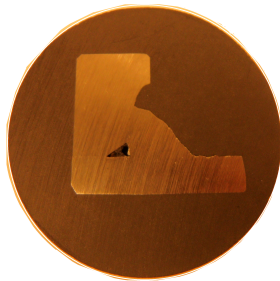
Figure 3.3: Bushing, shaft and disk sample in resin, Sample 1
