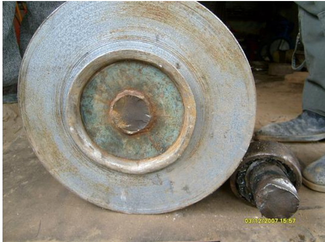
Figure 1.2: The fracture surface of a shaft. The turbine in the picture is another, larger model called Pamir Turbine. The failure is however the same for the HKT.
