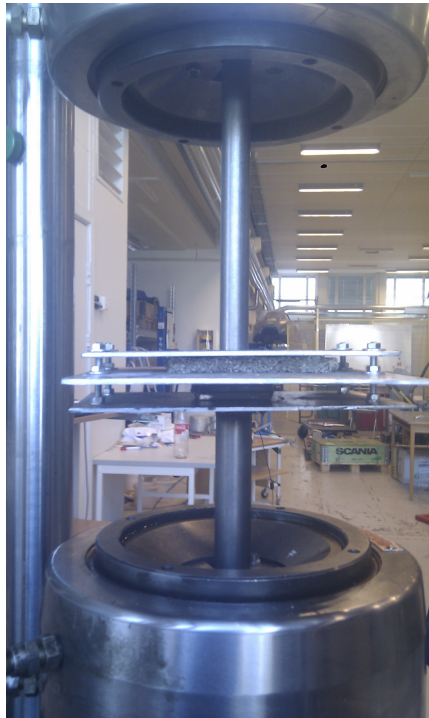
Figure 8.6: Reinforced test rig with sample
