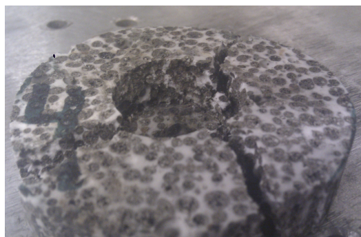
Figure 8.11: Specimen after shear testing
