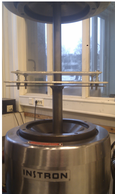
Figure 8.4: Punch tool lowered down through the guide and die
