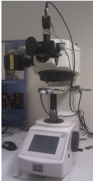
Figure 9.12: Test equipment for the vickers hardness test
