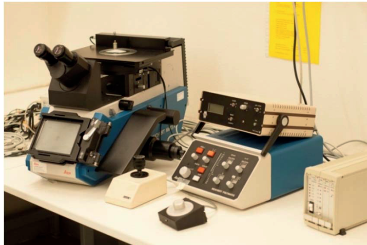
Figure 1: The imaging system used consists of an automated stage microscope (Reichert MeF3 A), a computer controlled automated stage control unit, manual control levers and a light source. The sideways-mounted Sony DXC 950P digital CCD camera is not visible in the picture.
