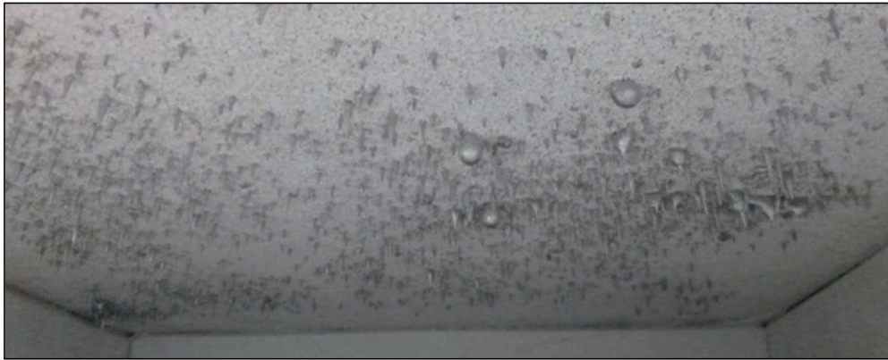
Figure 33: Solidified aluminium “needles” sticking out of the filters after a successful priming trial when starving the filter of metal and not submerging the filter in a metal bath. The present filter is a single 50 PPI CFF primed with 200 mm metal head. The metal was allowed to exit the filter box directly after the first metal penetrated through the filter. The weight of the filter after the trial suggests 96 % priming.
