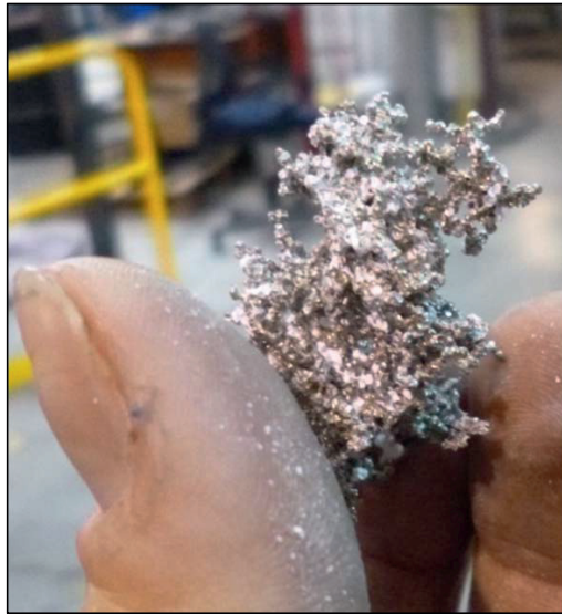
Figure 32: A piece of a primed 80 PPI CFF metal sample showing the fine anthill like structure. To secure the sample the CFF was chiselled out of the metal matrix.
