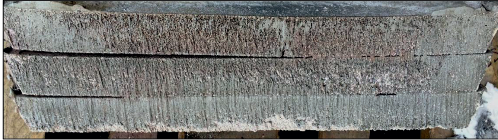
Figure 38: Fully Primed triple 50 PPI filter using the 23 inch filter system using pure aluminium with 1% Mg similar to a 3XXX series alloy. The filter has been starved with metal and therefore initiated draining prior the metal could fill the sump of the filter box. The filters have therefore not been submerged in metal. The samples have been cut by a waterjet cutting system, which makes the surface appear to be dull.
