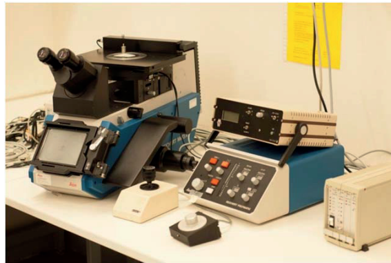
Figure 1: Automated stage microscope "Reichert MeF3 A". The computer controlled automated stage control unit, the manual control levers, the light source and its regulations and the microscope itself is shown in the image.
