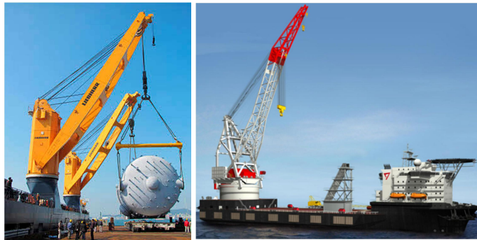
Figure 3.2 Lattice boom crane
