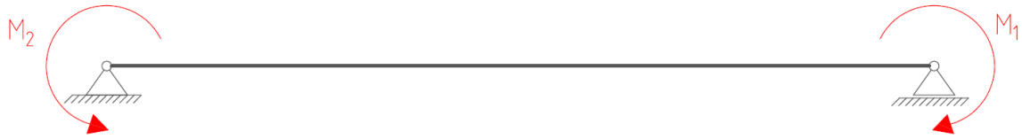
Figure 33: Hull beam support model with vertical bending moment applied at extremities. (Diewald, 2015)
