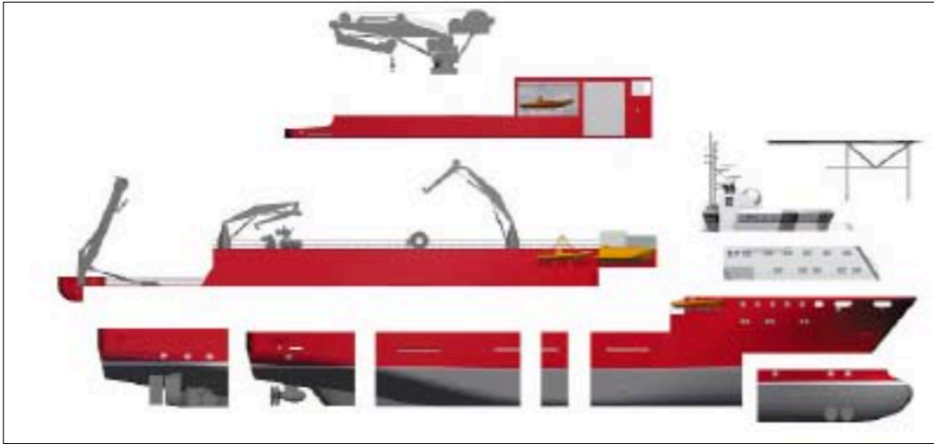
Figure 2-5 Ulstein has developed a modular production concept to achieve higher degree of standardization and efficiency in production (Erikstad & Levander, 2012)
