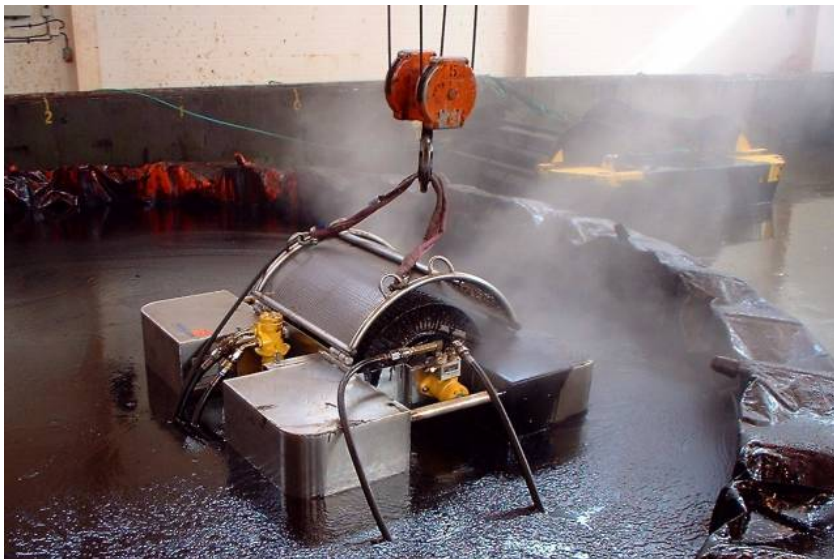
Bilde 15. Markleen MS 30 (Markleen Oil Spill Technology, 2006).
