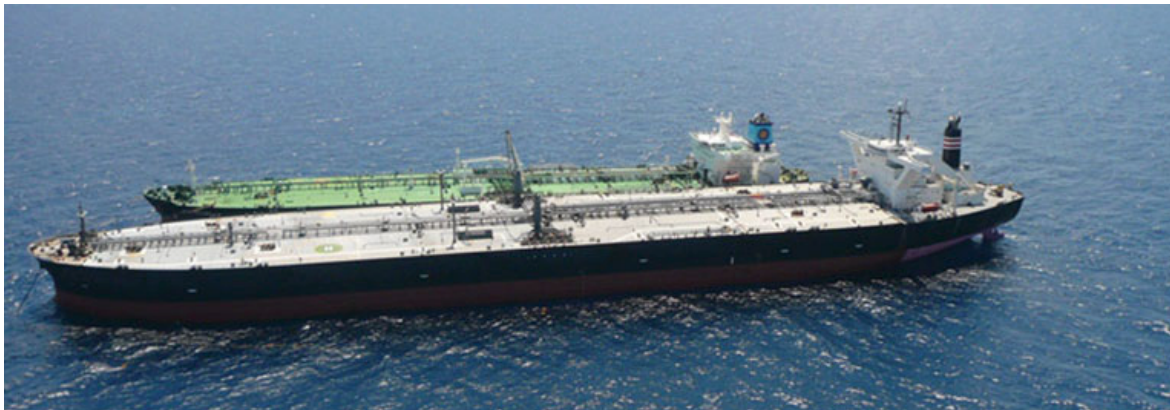
Bilde 2. STS-oljeomlasting (Fendercare marine, 2014).
