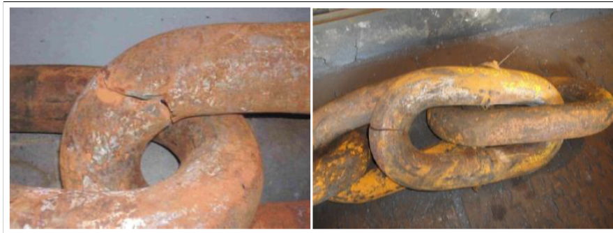
Figure 3.7: Examples of fractured chain specimens. The specimen on the left fractured at the bend, while the specimen on the right fractured at the crown.[Fernández et al., 2014, p.4].
