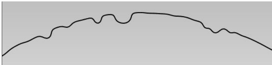
(a) Extracted profile from corrosion on chain specimen.
