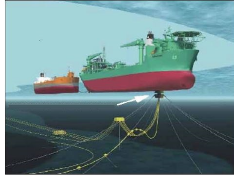
Figure 2.4: Single Point Mooring. Adapted by author from (Noble Denton Europe Limited, 2006, p. 22).
