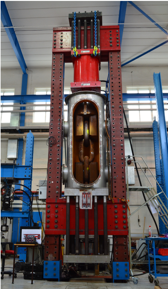
(a) Fatigue testing machine. The grey chamber was filled with saltwater during testing.
