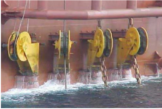
Figure 2.3: Spread Mooring. Adapted by author from (Noble Denton Europe Limited, 2006, p. 26).
