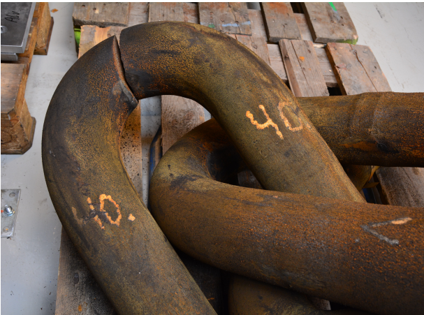
(c) Failure in the crown region of a tested chain link.
