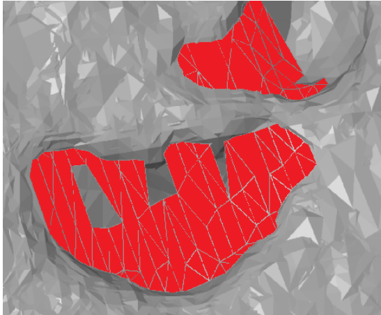
Figure 6.9: Due to measuring errors, some cavities got "filled up" in the resulting triangle mesh.
