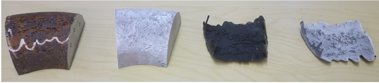
Figure 6.3: The four test objects assessed, from left to right: TO1 with original chain surface, TO2 with coloured chain surface, TO3 as cast with original surface color and TO4 as cast with coloured surface.
