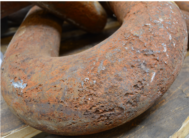
(b) Surface condition of a retrieved link.
