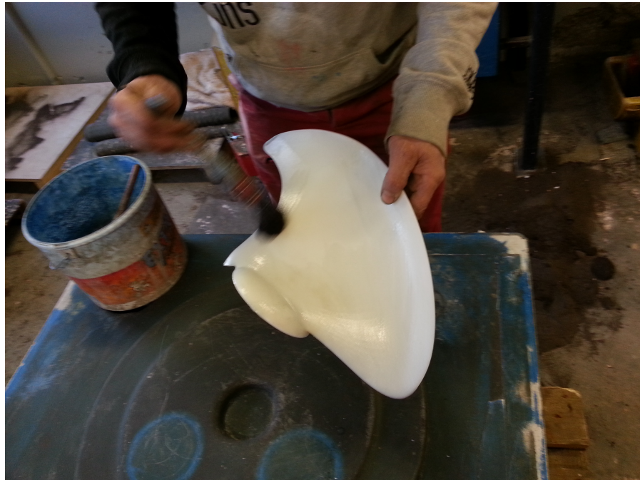
Figure 4: Slip coating to ease pattern removal from mold.
