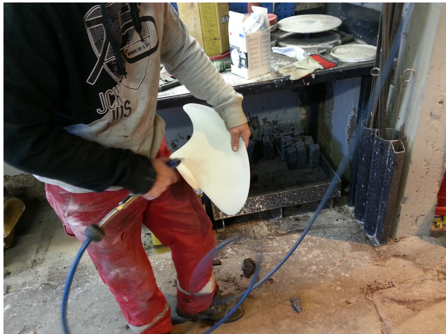
Figure 5: Air Drying of Slip coat.
