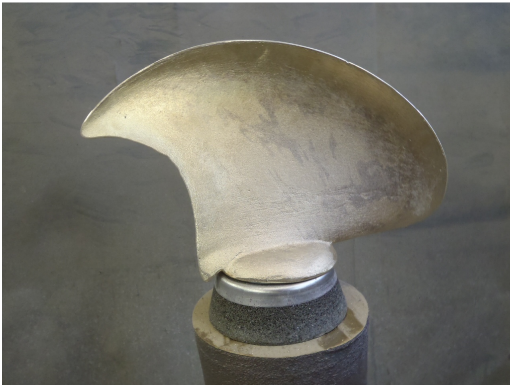
(b) Resulting Cast with gating system removed.
