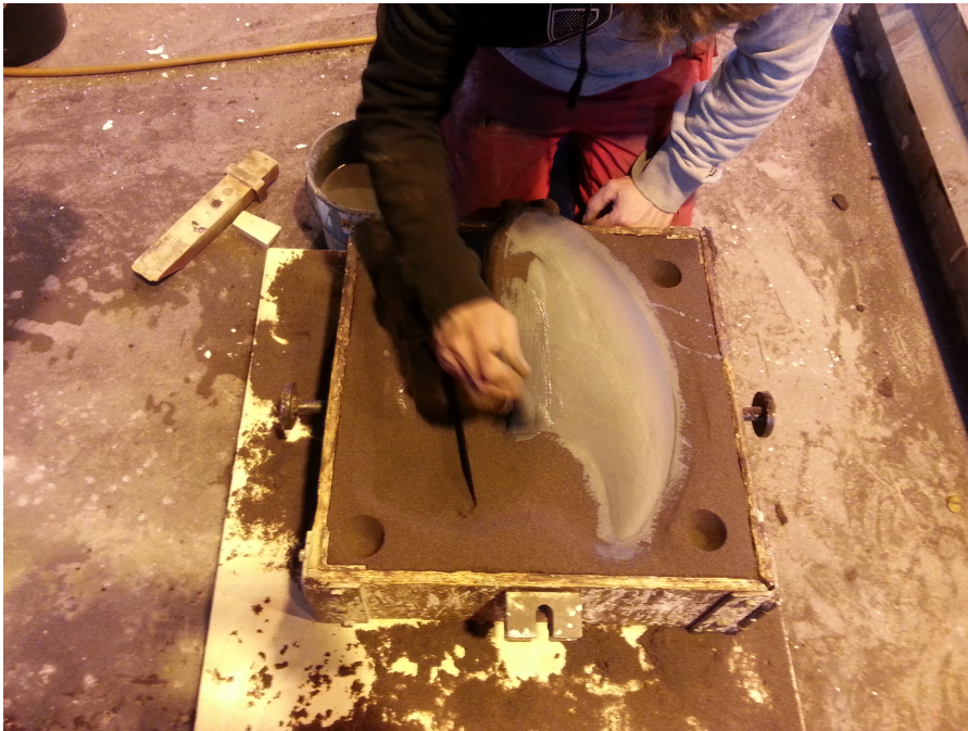
Figure 9: Coating of the cope and drag.
