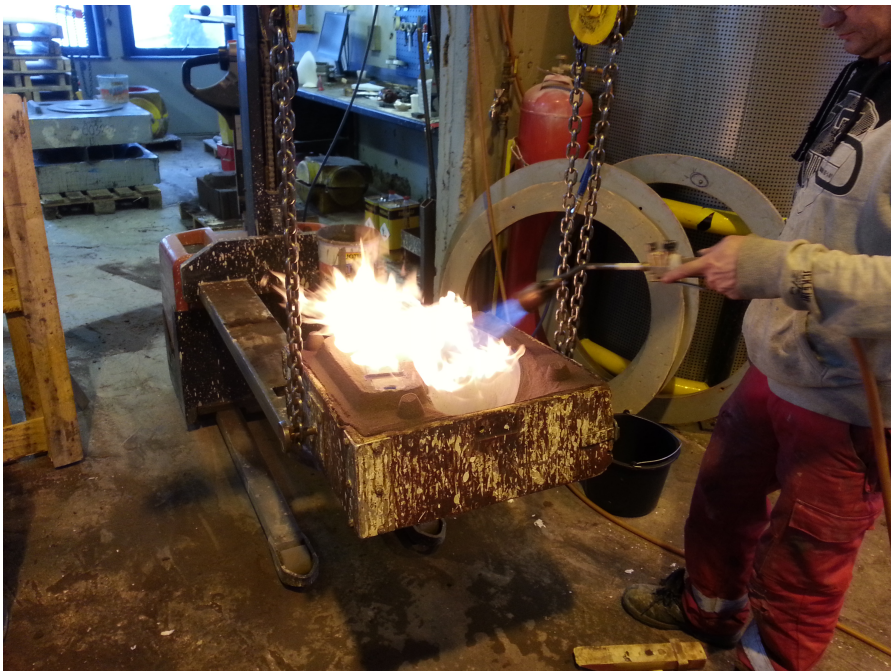
Figure 10: Burning of residue to remove moisture from mold.
