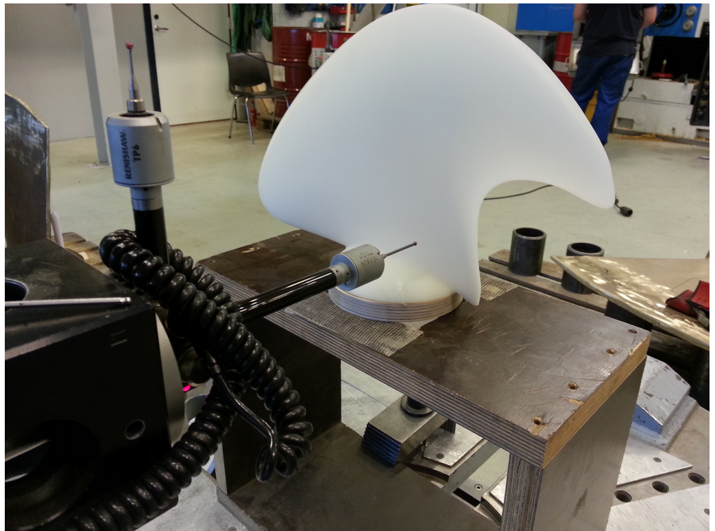
(b) Model being measured for dimensional accuracy.
