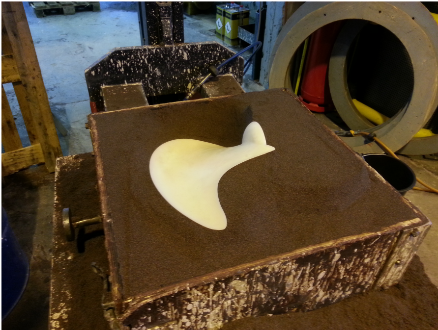
Figure 6: Creating the cope and drag.
