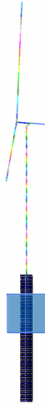
Figure 7.2: The model in FEDEM. The monopile is indicated as the visualized structure
