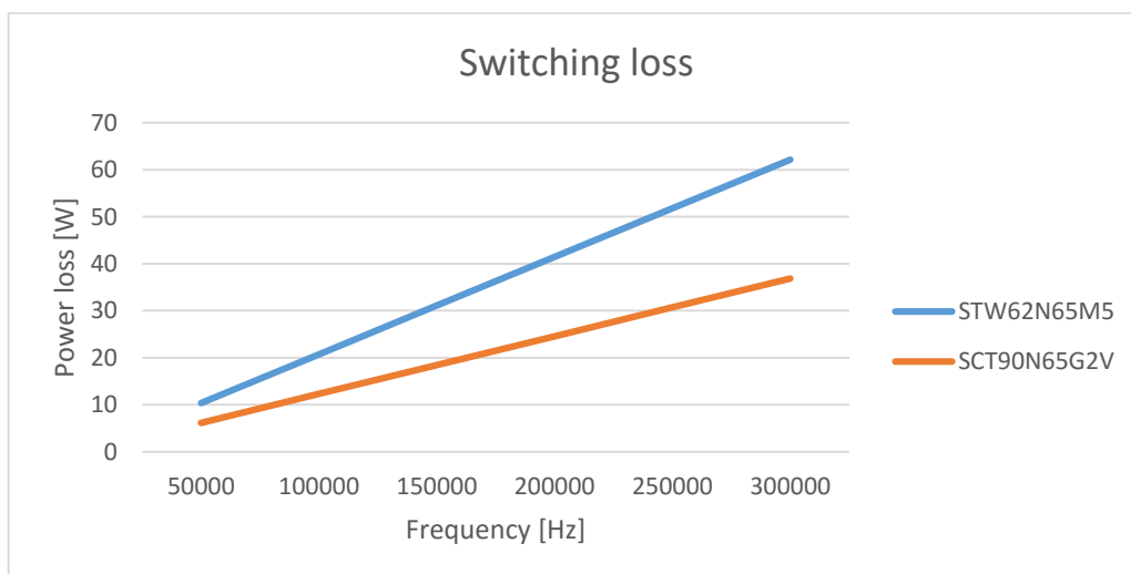
Figure 22: Calculated switching loss from datasheet energy loss
