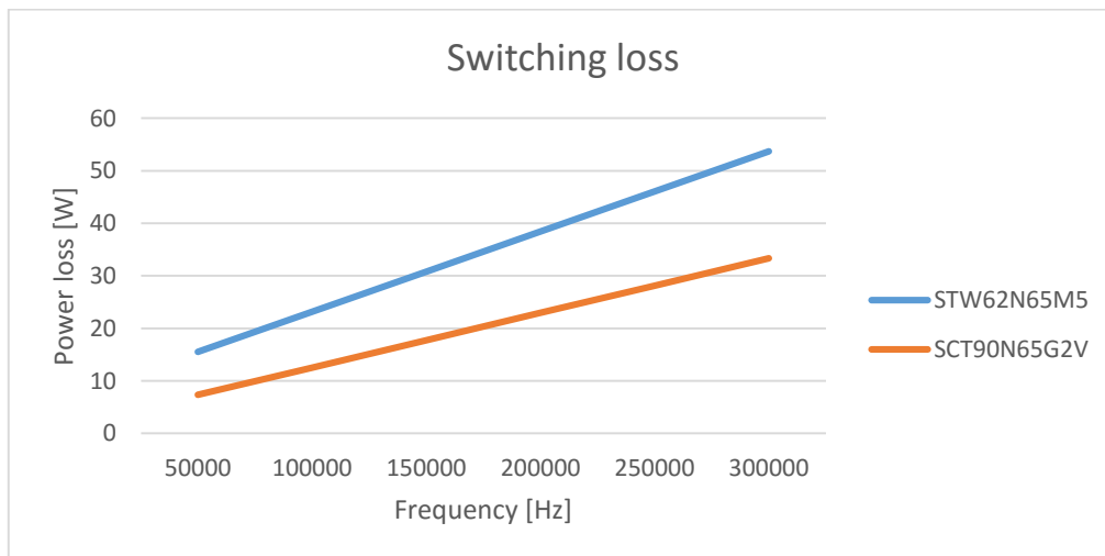
Figure 23: Calculated MOSFET power loss from Equation 20.
